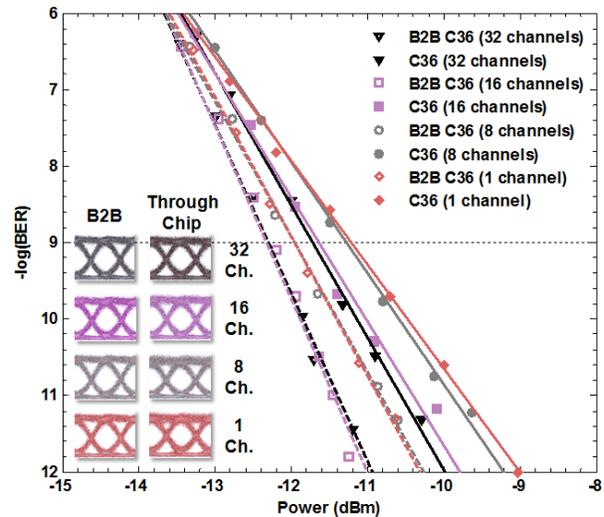
Fig. 4: BER curves measured on wavelength channel C36 when 1, 8, 16, and 32 wavelength channels are on, showing a  $0.65 \pm 0.08$  dB power penalty, and an inset of back-to-back and output eye diagrams.
