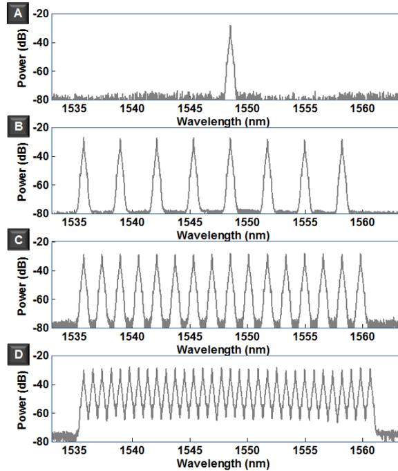
Fig. 2: a-d. OSA traces recorded after propagation through the silicon photonic chip, depicting experimental configurations with 1, 8, 16, and 32 modulated wavelength channels.
