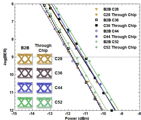
Fig. 3: BER curves for C28, C36, C44, and C52, showing a constant  $0.58 \pm 0.07$  dB power penalty, and an inset of output eye diagrams including the back-to-back case.
