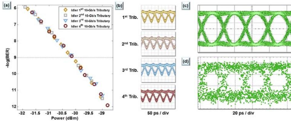
**Fig. 2:** a. BER measurements of the 10-Gb/s tributaries. b. Idler eye diagrams recorded at the inverted-data differential output port of the APD. c. 40-Gb/s Electrical eye diagram recorded directly from the PPG. d. 40-Gb/s eye diagram reconstructed from the optical sampling process by sweeping the pump pulse timing (recorded at the APD's output).
