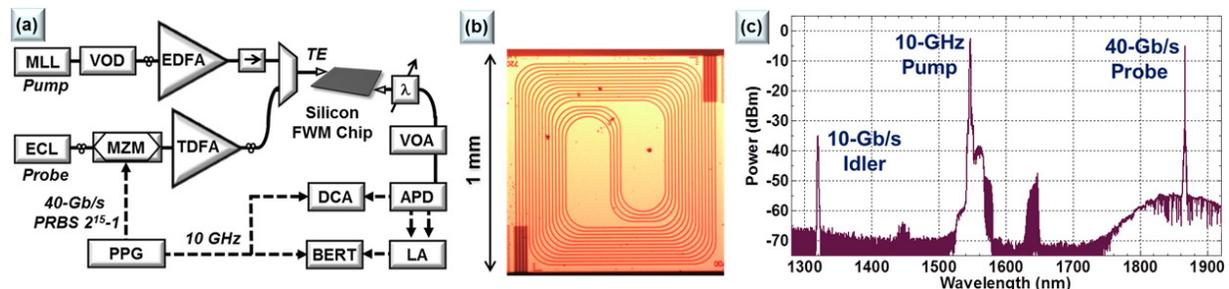
Fig. 1: a. Experimental setup. b. Microscope image of the silicon nanowaveguides. c. OSA trace recorded at the chip's output.
