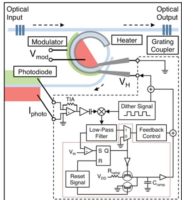
**Fig. 2:** The device used in this experiment (not to scale). The off-chip electronics interfacing with the integrated photonic elements are shown in the dashed box. Highlighted in red is the circuitry devoted to wavelength locking.
