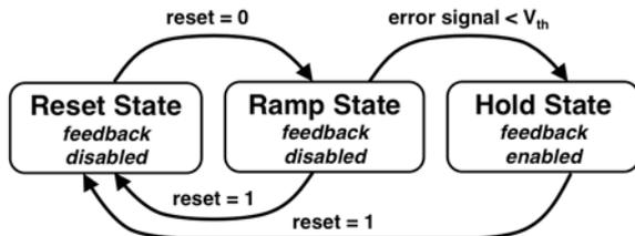
**Fig. 3:** A state diagram describing the functionality of the wavelength-locking circuitry (dashed red box, Fig. 2)
