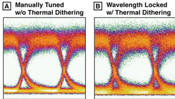
**Fig. 5:** A comparison between (a) manually tuning the integrated heater to achieve an optimum modulation and (b) using the wavelength locking system to tune the integrated heater automatically.
