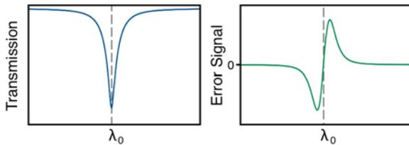
**Fig. 1:** The optical resonance of a microring resonator (left) and the error signal generated when applying a dithering signal to the microring resonator (right).
