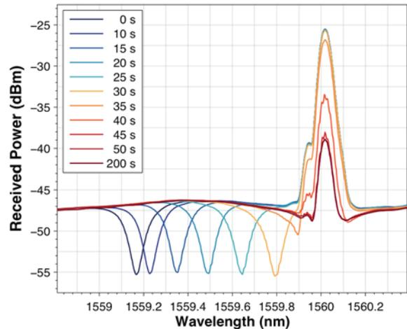
**Fig. 4:** Optical traces show the microring resonance being tuned and wavelength locked to a laser source.
