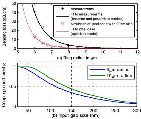
**Fig 1:** a) Bending loss measured and simulated in<sup>4</sup> for various radii, and associated power law fits used in the three defined ring loss models. b) Impact of input gap size on coupling coefficient.
