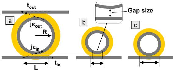
**Fig 2:** Impact of radius and gap size on coupling length  $L$ . a) and b) have same gap sizes but the smaller diameter of b) results in a shorter approximated coupling length. b) and c) are of equal diameter but different gap sizes, resulting in different coupling lengths, and distinct coupling coefficients  $\kappa$  and  $t$ .
