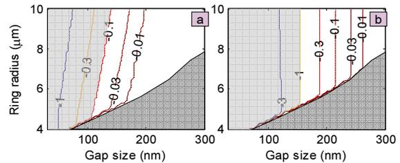
**Fig 4:** a) Insertion loss for non-dropped signals ( $\text{IL}_{\text{thru}}$ ), at  $\text{FSR}/2$ , in dB b) Insertion loss for frequency showing a  $1\text{nm}$  detuning with resonant frequency, in dB.
