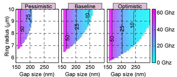
**Fig 5:** Regions of interest with different ring loss models. Designs leading to unacceptable insertion losses have been removed. Color reflects  $3\text{-dB}$  bandwidth of the ring.
