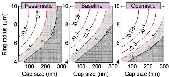
**Fig 3:** Insertion loss (dB) at resonant frequency ( $IL_{drop}$ ), for various ring designs, and considering three loss models.
