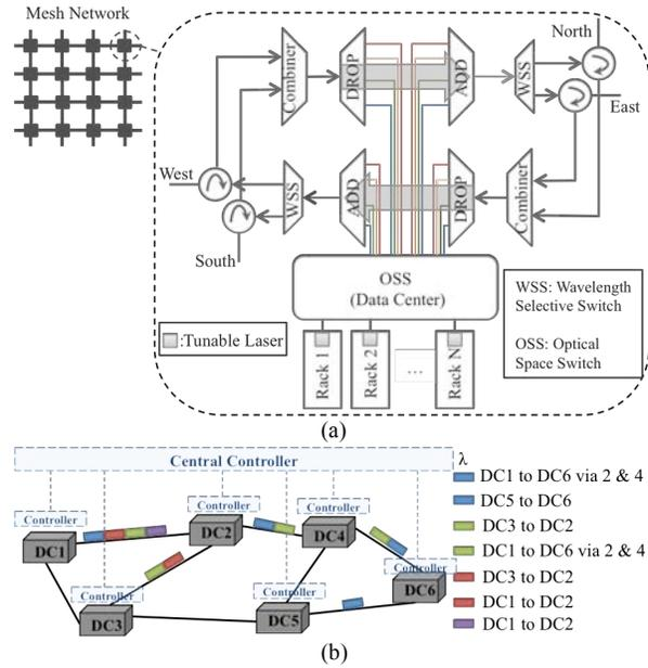
Figure 1: (a) 2x2 bidirectional software-defined optical gateway in a mesh network. The OSS provides the switching substrate for both inter and intra connectivity, (b) An example of wavelength assignment in the transport network across data centers by the distributed controller.
