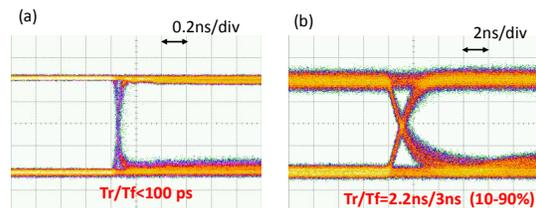
Fig. 3. (a) Electrical input voltage to the p-i-n junction of the switch. (b) Optical output of the switch.
