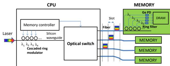
Fig. 1. An optically connected memory system composed of silicon photonic devices.
