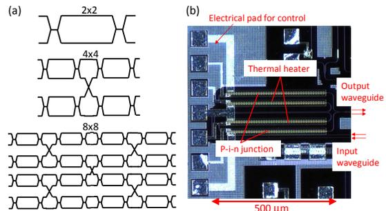
Fig. 2. (a) Structures of cascaded MZI switches. (b) A photograph of the 2×2 silicon photonic switch utilized in this measurement. A thermal heater and a built-in p-i-n junction are fabricated on each arm.
