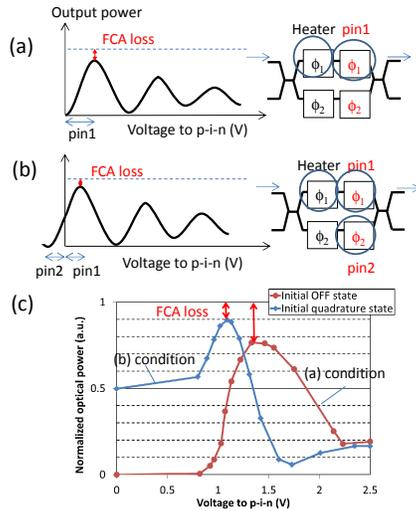
Fig. 4. Output powers of the 2x2 MZI switch. (a) Operating with a single p-i-n junction. Initial phase is adjusted to OFF state. (b) Operating with two p-i-n junctions. Initial phase is adjusted to quadrature state. (c) Measured FCA loss with different operating conditions.
