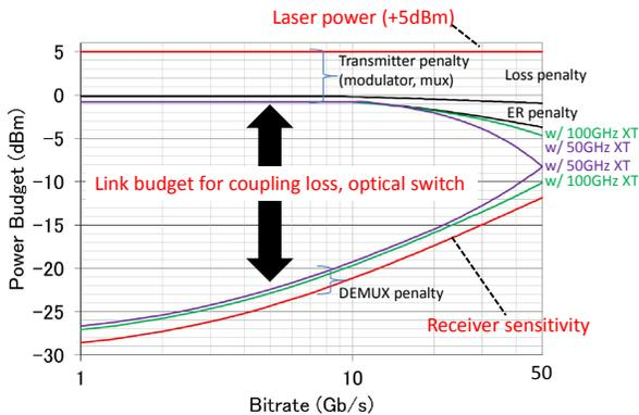
Fig. 5. Silicon photonic link power budget calculated from model of cascaded ring modulator, cascaded ring demultiplexer and receiver with germanium photodiode.
