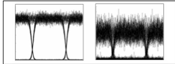
**Figure 3.** Eye diagrams of the simulated input and output signals after propagation through 20 nodes.
