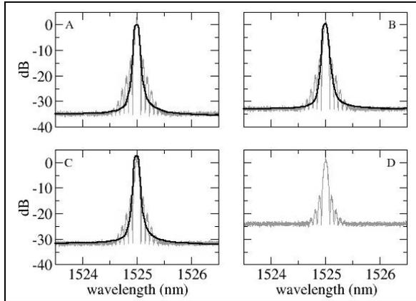
**Figure 2.** Panel A illustrates the experimentally-observed (dark) and simulated (light) input spectra; Panels B and C compare these spectra after one and two nodes, respectively. Panel D presents the projected spectrum after propagation through 20 nodes.
