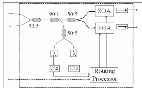
Figure 1. Schematic of a single Data Vortex switching node (after [2-4]).
