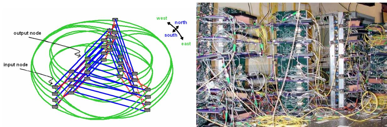
Fig. 1. Graphical depiction of the implemented  $12 \times 12$  Data Vortex topology which contains 3 cylinders, each with 4 nodes in the height dimension and 3 nodes in the angular dimension. Photograph of implemented system (right pane).
