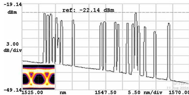
Fig. 5. Spectrum of the 14-payload channel 5-header optical packets (the frame and header wavelengths have higher peak powers). Eye diagram of the payload channel at 1564.7 nm confirms the measured BER of  $10^{-9}$  at 10 Gbps (inset).
