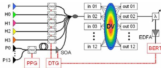
Fig. 3. Schematic of the experimental setup containing the implemented Data Vortex switching fabric and the necessary input signal modulation (PPG: 10-GHz pulse pattern generator; DTG: low-speed data timing generator).
