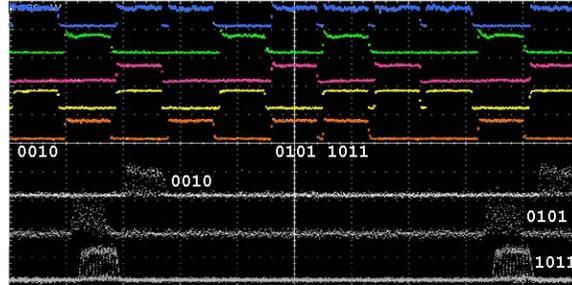
Fig. 4. The frame and header signals of the eight packets, followed by the emerging packets' payload waveforms.
