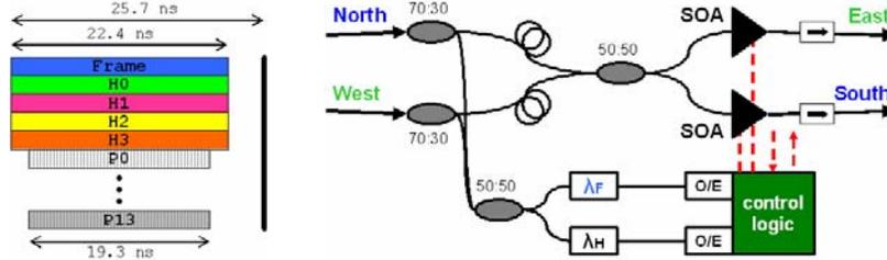
Fig. 2. Diagram of the DWDM header-parallel encoded packet format (left pane). Schematic of a Data Vortex switching node (right pane), containing fiberoptic couplers, filters ( $\lambda$ ), photodetectors (O/E), and isolators (arrows).
