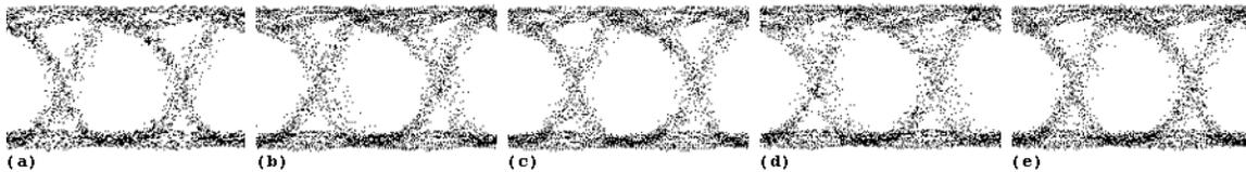
Fig. 5. Electrical eye diagrams of 10 Gbps signal on 1546.92 nm (C38) at (a) the system input and system output for (b) 4-, (c) 8-, (d) 12-, and (e) 16-wavelength packets.
