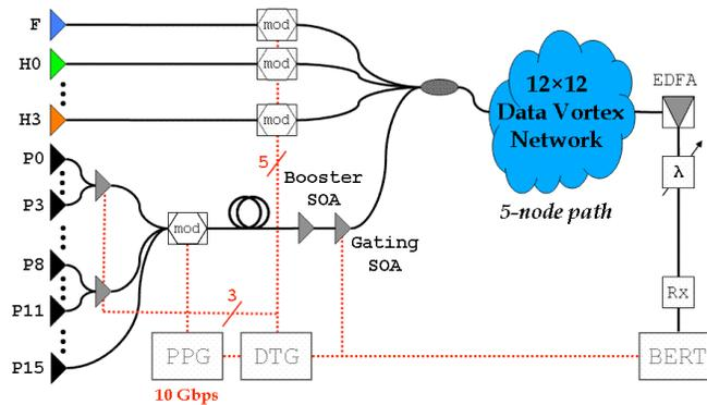
Fig. 3. Schematic of the experimental setup containing the implemented  $12 \times 12$  data vortex switching fabric and the necessary input signal modulation with a PPG (pulse pattern generator) and DTG (data timing generator). At the output, one payload wavelength is selected by the tunable filter for gated BER measurement.
