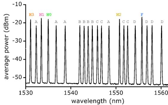
Fig. 4. Plot of the spectrum of the injected packets. *F* and *H0* through *H3* designate the parallel header wavelengths while the labels *A*, *B*, *C*, and *D* indicate the grouping of the payload wavelengths.
