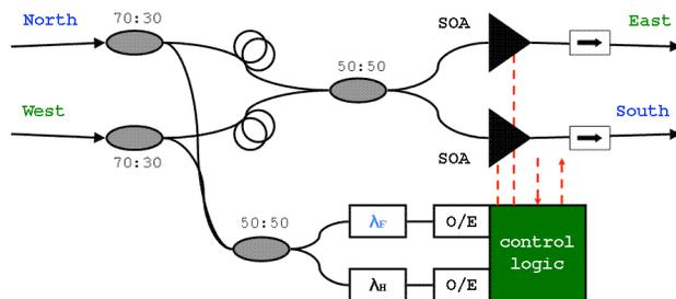
Fig. 1. Schematic of the photonic switching node design (ovals for optical couplers,  $\lambda$  filters, O/E photodetectors, and boxed arrows for isolators, dashed arrows for deflection signal input and output).
