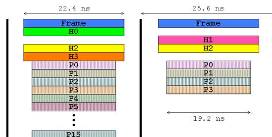
Fig. 2. Illustration of the multiple-wavelength packet format, with constant-value wavelength-parallel header bits. The left packet contains the maximum of 16 payload wavelengths (384 B), while the right one contains just 4 payload wavelengths (96 B).
