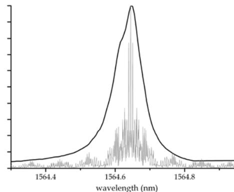
Fig. 2. Plot of the ring resonator wavelength response with the power spectrum of a 10 Gbps PRBS signal superimposed.
