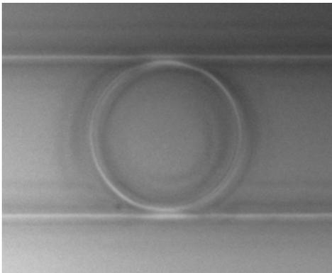
Fig. 1. Micrograph of the ring resonator device, which has a diameter of 10  $\mu\text{m}$  and a waveguide–ring gap of 200 nm.
