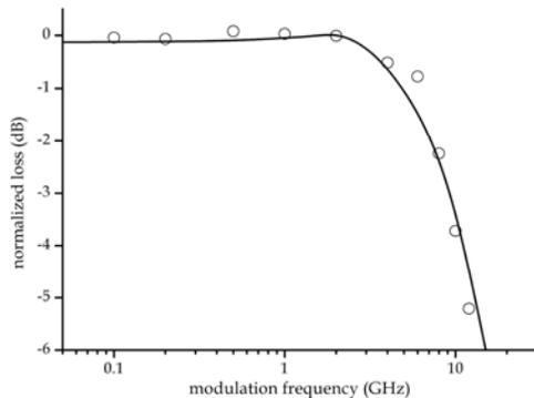
Fig. 3. Amplitude Bode plot for the ring resonator's drop port, including both experimentally measured ( $\circ$ ) and numerically simulated ( $\text{—}$ ) data.
