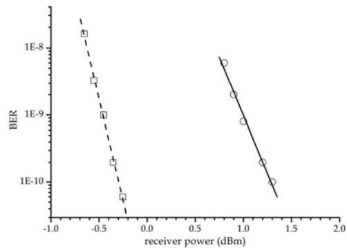
Fig. 4. Plot of BER as it varies with receiver power for the through port ( $\square$ ; back-to-back case) and for the drop port ( $\circ$ ). The receiver power penalty is accordingly determined to be  $1.4 \pm 0.1$  dB.
