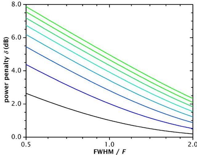
Fig. 6. Plots of power penalty versus the ratio of FWHM (in gigahertz) to modulation frequency  $F$  (in gigabits per second), for a single microring resonator (black) and cascades of two through eight microrings (blue to green), obtained from the numerical model discussed in Ref. [27].
