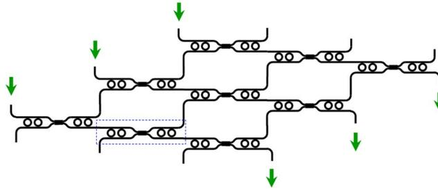
Fig. 1. Conceptual illustration of an augmented  $3 \times 3$  crossbar network, with a single multiple-wavelength electrically controlled nonblocking switching element highlighted. The coupled waveguides in each switch implement a crossover, and the microring resonators on the same half of the switching elements operate on staggered wavelengths in order to further enhance the bandwidth.
