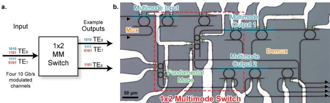
Fig. 1. (a) Block diagram of 1x2 multimode switch operation. The example shows three channels routed to Output 1 and one channel to Output 2. (b) Optical microscope image of fabricated device. The areas highlighted in blue show the multimode waveguides, which transition to single-mode by adiabatic tapering. In order to couple on and off the chip using single-mode edge coupling, its multimode input is preceded by a multiplexer and each output uses a demultiplexer.
