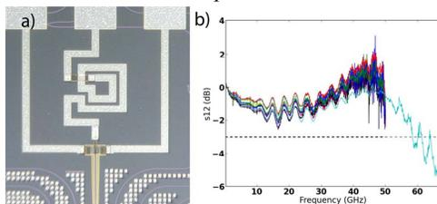
Fig. 2. (a) Micrograph of gain-peaked photodetector. (b) EO response of a several photodetectors up to 50 GHz and a single high-speed measurement showing 58 GHz bandwidth.
