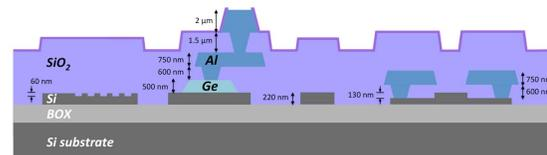
Fig. 1. Cross section of grating couplers, photodetectors, waveguides, and modulators available in the platform.
