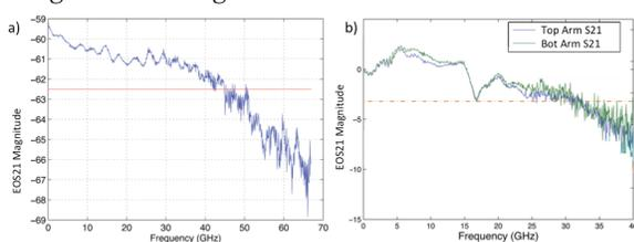
Fig. 3. Typical EOS21 performance of the (a) ring and (b) TWMZ devices showing 3dB bandwidths of 40 and 30 GHz, respectively.
