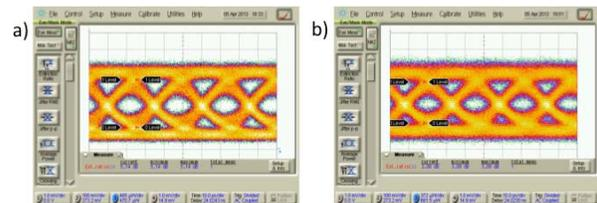
Fig. 4. 40Gb/s Eye-diagrams of a differentially-driven TWMZ with: (a) 0.25 V bias and 2.5 V<sub>pp</sub> drive voltage, (b) 0 V bias and 1.6 V<sub>pp</sub> drive voltage.
