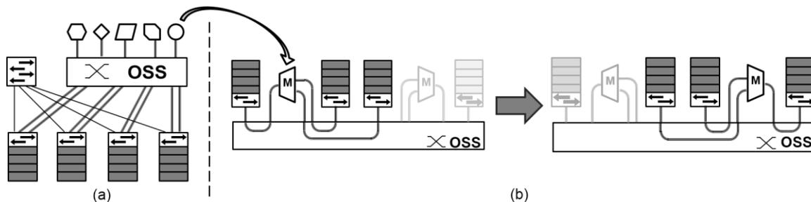
Fig. 1. (a) Hybrid network architecture featuring various photonic capabilities, as represented by the polygons. (b) Utilizing the optical space switch to dynamically deliver optical layer multicast between different racks in a data center.
