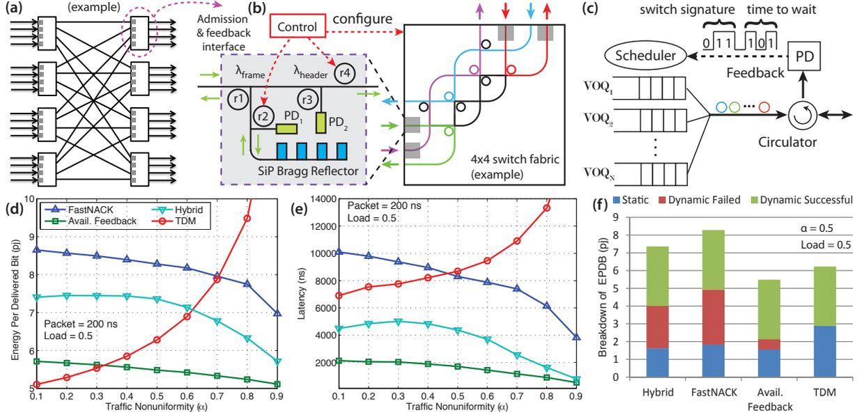
Fig. 1. (a) An example multistage interconnect formed by (b) an example  $4 \times 4$  SiP switch element incorporated with the admission and feedback interface; (c) client Tx interface; (d) energy efficiency and (e) latency versus traffic nonuniformity  $\alpha$ ; (f) energy profile when  $\alpha = 0.5$ .
