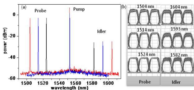
Fig. 3 (a) Overlaid Spectra of wavelength conversion recorded directly after the chip. Probe wavelengths are set to 1504, 1514, and 1524 nm, respectively. (b) Eye diagrams of back-to-back (probe) and wavelength converted signals (idler) with different probe-idler separations.
