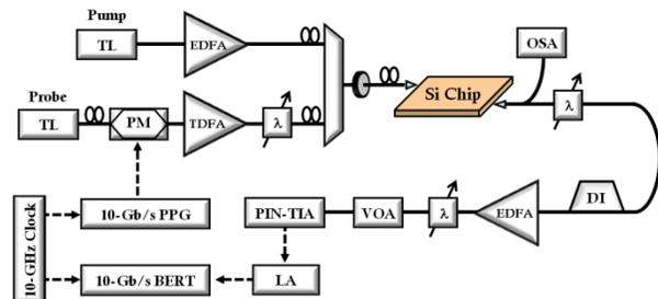
Fig. 1 Diagram of experimental setup.
