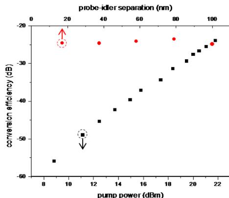
Fig. 2 Conversion efficiency versus probe-idler wavelength separation with a pump wavelength of 1552.5 nm and a pump injection power of 21.5 dBm (red dots); Conversion efficiency as a function of injected pump power with 1552.5-nm pump and 1504-nm probe (black dots).
