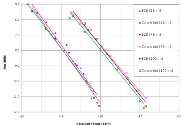
Fig. 4 10-Gb/s BER curves of back-to-back and wavelength-converted signals with constant 1-dB power penalties for probe-idler separations of 58, 79, and 100 nm.
