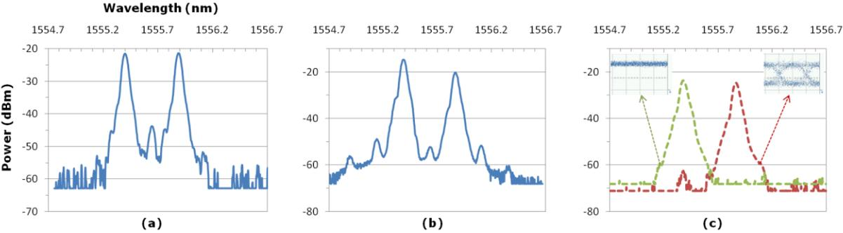
Fig. 3 spectrum of (a) before the silicon chip (b) after the chip (c) filtered sideband. Inset: waveform of the sideband in time domain.
