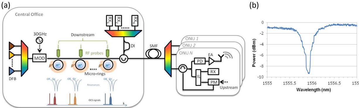
Fig. 1 (a) Architecture of wired and wireless networks using single sideband modulation with colorless ONU. Inset: conceptual diagram of single sideband modulation. (b) Spectrum of the microring in its passive state.
