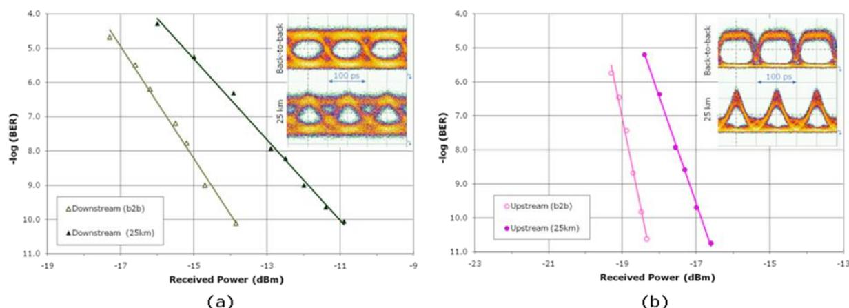
Fig. 4 BER measurement of (a) downstream NRZ signals (b) upstream DPSK signals. Inset: respective eye diagrams.
