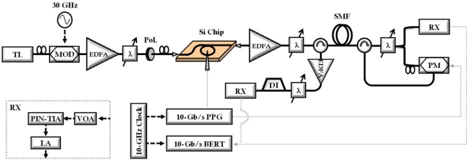
Fig. 2 Experimental setup. Inset: optical receiver.
