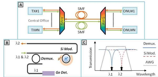
Fig. 1. (a) Architecture of the proposed WDM PON. (b) Configuration of the individual colorless ONU. (c) Transmission spectra of the AWG, microring demultiplexer (Demux), and the microring modulator (Si Mod.), respectively.
