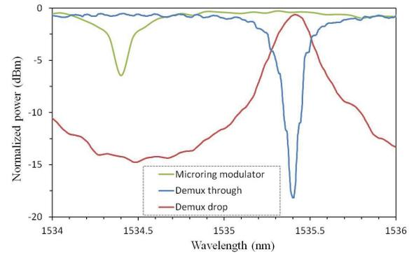
Fig. 3. Measured spectra of the microring demultiplexer and modulator.
