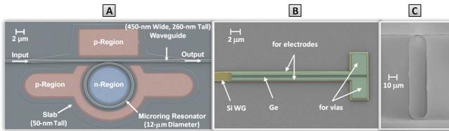
Fig. 2. Scanning-electron-microscope (SEM) image of (a) modulator, (b) photodetector, and (c) demultiplexer.
