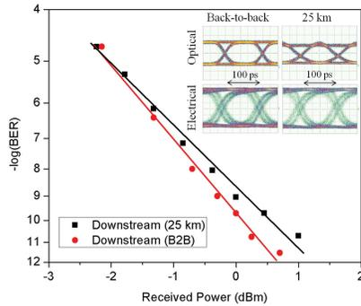
Fig. 5. BER measurement of the 10-Gb/s downstream signal. Inset: optical and electrical eye diagrams of the back-to-back and 25-km fiber transmission case.
