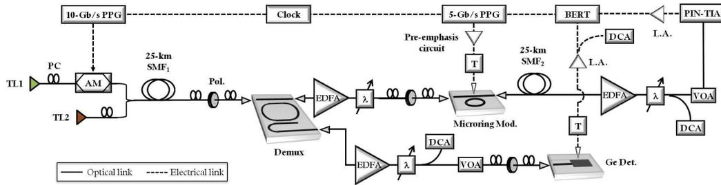
Fig. 4. Experimental setup.
