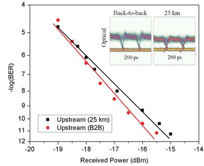
Fig. 6. BER measurement of the 5-Gb/s upstream signal. Inset: optical eye diagrams of the back-to-back and 25-km fiber transmission case.
