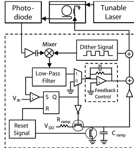
Fig. 1. Schematic of the experimental setup and the wavelength initialization circuitry, with configuration of the chip indicated in top-center of the diagram.
