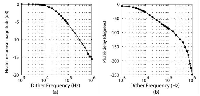
Fig. 5. (a) Heater modulation magnitude and (b) phase response as dithering frequency is increased.
