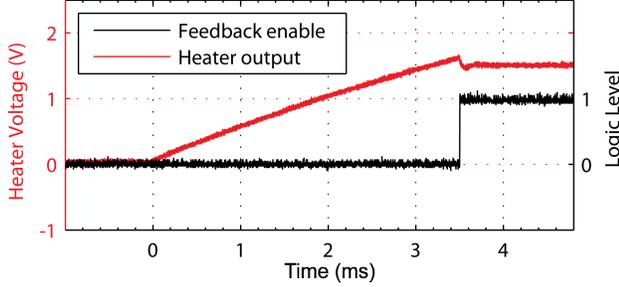
Fig. 2. Voltage applied to heater during the initialization process.
