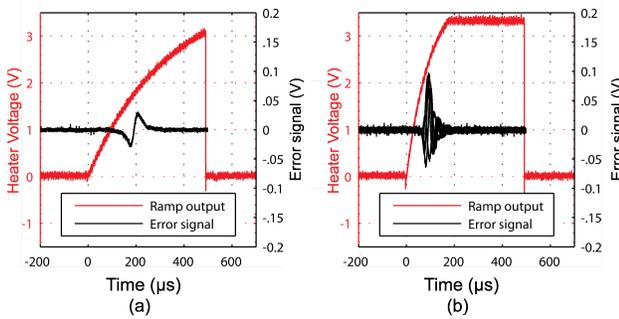
Fig. 3 (a) A fast heater ramp signal generating a usable error signal. (b) A ramp signal that is too fast and generating an unstable error signal.
