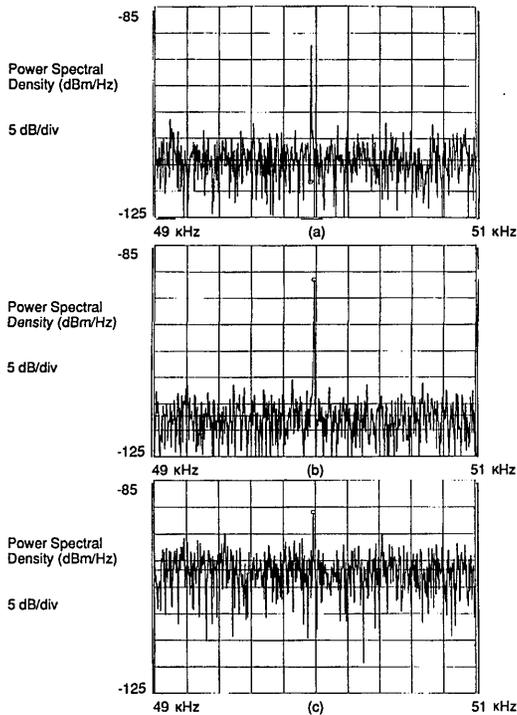
Fig. 4. Experimental results demonstrating signal-to-noise ratio improvement beyond the shot-noise limit. (a) The 50-kHz signal with shot noise, (b) the same signal measured with squeezed noise projection for 3-dB improvement, (c) the signal immersed in 12 dB of (excess) antisqueezing noise.
