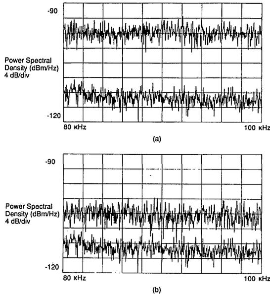
Fig. 2. Power spectra from the balanced detection showing cancellation of excess phase noise. In (a) the maximum projected noise is the sum of antisqueezing and the GAWBS; in (b) with the  $\pi$ -phase-modulation scheme 8 dB of GAWBS noise is canceled.
