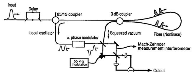
Fig. 3. Configuration used for the sub-shot-noise phase measurement at 50 kHz. The reflected pump is partly reused as the measurement probe in a Mach-Zehnder interferometer.
