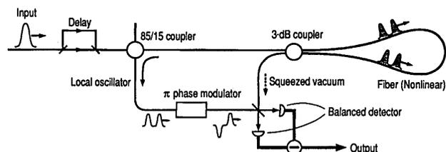
Fig. 1. Experimental configuration of the scheme used to cancel the GAWBS-induced phase noise. Two consecutive pulses delayed by 500 ps enter the fiber ring. One pulse is  $\pi$  phase shifted with respect to the second pulse in the local-oscillator path.
