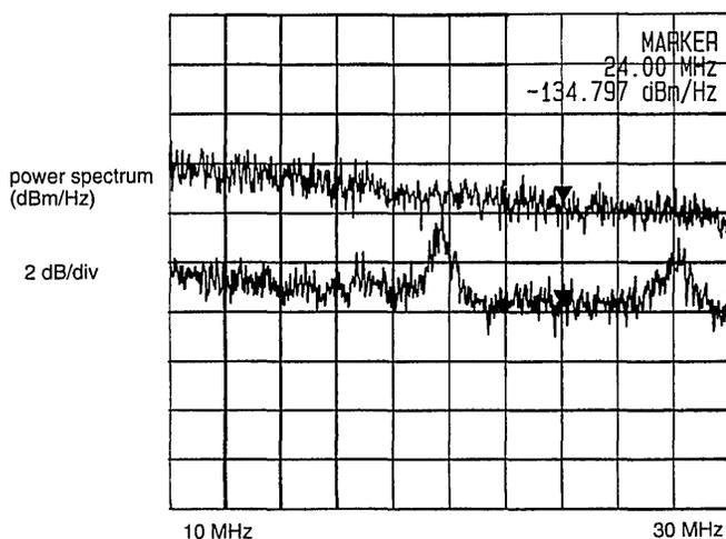
Fig. 5. Squeezing measured between GAWBS peaks from 10 to 30 MHz with 440 mW of average power. The upper curve is the shot-noise level, and the lower curve is the squeezed-noise level. At frequencies corresponding to GAWBS excitations the squeezing is destroyed.
