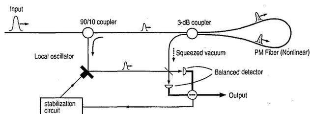
Fig. 2. Experimental configuration used to measure squeezing with a 1-GHz pump.
