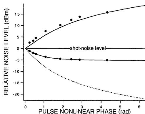
Fig. 4. Squeezing and antisqueezing magnitudes (filled circles) measured between 80 and 100 kHz for a range of input average powers (maximum was 440 mW) plotted along the analytical predictions with the assumptions of Gaussian pulse shape and 85% detection quantum efficiency (solid curves). The dashed curve is the expected optimum squeezing with perfect detection and ideal local-oscillator phase bias.
