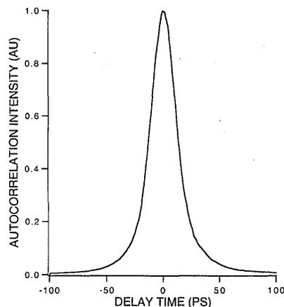
Fig. 1. Autocorrelation trace of the gigahertz source output pulse. The FWHM is 15 ps, assuming a sech profile.
