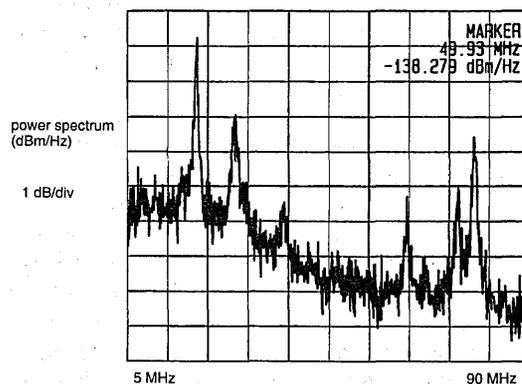
Fig. 3. GAWBS power spectrum (shown from 5 to 90 MHz) obtained with the balanced homodyne receiver by measurement of the amplified noise quadrature. The input average power of the 1-GHz mode-locked pulses is 20 mW.
