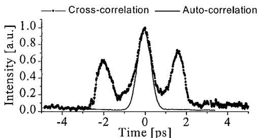
Fig. 5. Autocorrelation and cross correlation between adjacent pulses.
