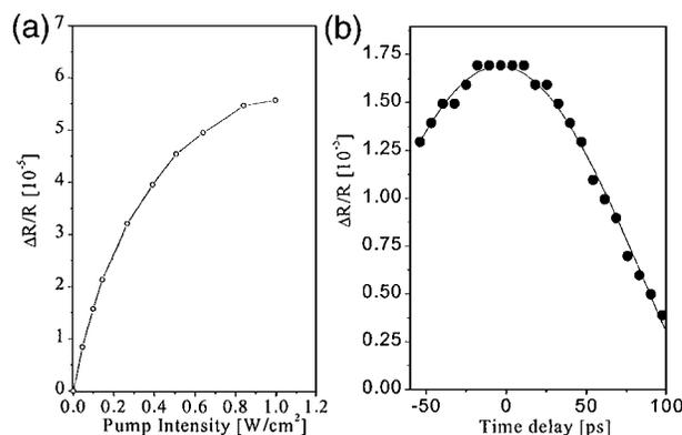
Fig. 1. Change in reflectivity as a function of (a) 1480-nm power density and (b) delay between the modulated 1480-nm pump and the 1550-nm pulses.
