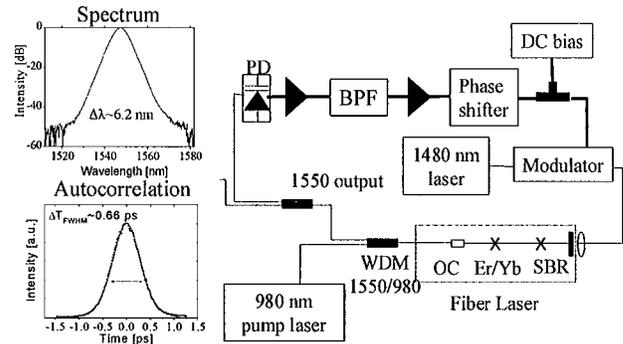
Fig. 2. Diagram of the fiber laser and the optical feedback loop. Top inset, laser spectrum; bottom inset, laser pulse autocorrelation. PD, photodiode; WDM, wavelength-division multiplexer; OC, output coupler.
