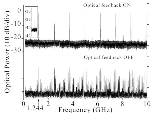
Fig. 3. rf spectra of the laser output with the optical feedback on and off. The fundamental mode of the cavity is suppressed by  $\sim 37$  dB (see inset).
