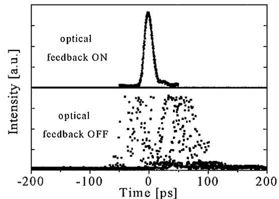
Fig. 4. Fast digital scope traces of the laser output with the optical feedback on and off.
