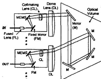
Fig. 1: Schematic of modular optical system.
