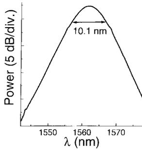
Fig. 7. Optical spectrum of the laser operating at 155 MHz. The FWHM is indicated.
