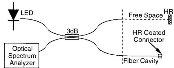
Fig. 12. Schematic of the Michelson interferometer used to measure cavity dispersion.
