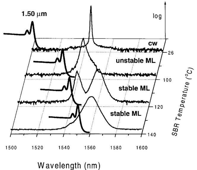
Fig. 4. Optical spectrum (thin line) of laser output and approximate exciton absorption (thick line) for various temperatures of the SBR.
