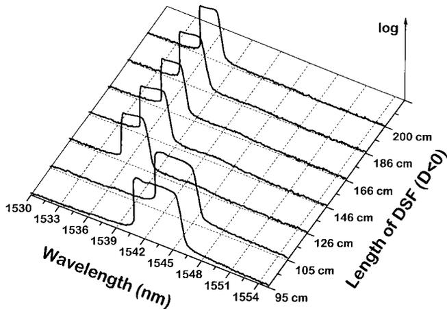
Fig. 5. Optical spectra of the pulses generated with the laser operating in the normal dispersion regime for different lengths of DCF.
