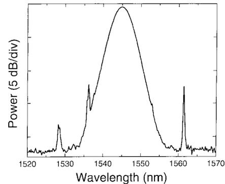
Fig. 6. Optical pulse spectrum of the fiber laser output with resonance sidebands present.
