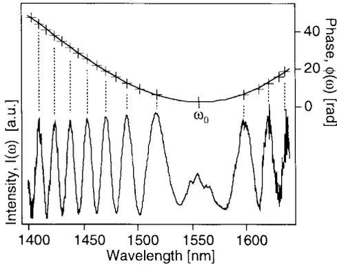
Fig. 13. Typical normalized optical spectrum measured out one port of the interferometer is shown in the bottom curve. The plot of the associated phase (crosses) created by locating each peak and valley of the normalized spectrum and assigning the proper phase value is shown. The fit of the theory used to determine  $\beta_2$  is superimposed (solid line).
