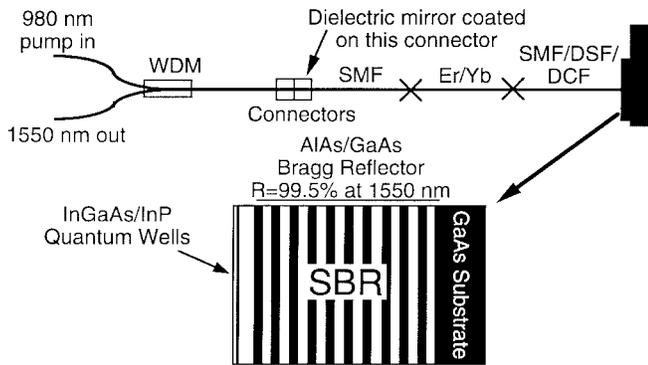
Fig. 1. Schematic of the fiber laser cavity and structure of the SBR.
