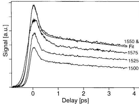
Fig. 3. Pump-probe response of the SBR indicating the relative change in the reflectivity at several wavelengths. The theoretical fit to the response at 1550 nm is superimposed (see Section VI).
