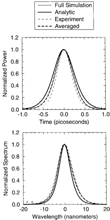
Fig. 9. Steady-state pulse profiles and optical spectra given by (1)–(4) and comparison of this model with the averaged model, the analytic approximation and the experimental findings.
