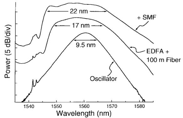
Fig. 10. Optical spectra from bottom to top: output of oscillator, after amplifier and 100 m of low normal dispersion fiber and after further propagation through SMF fiber. Spectra are offset vertically for clarity.
