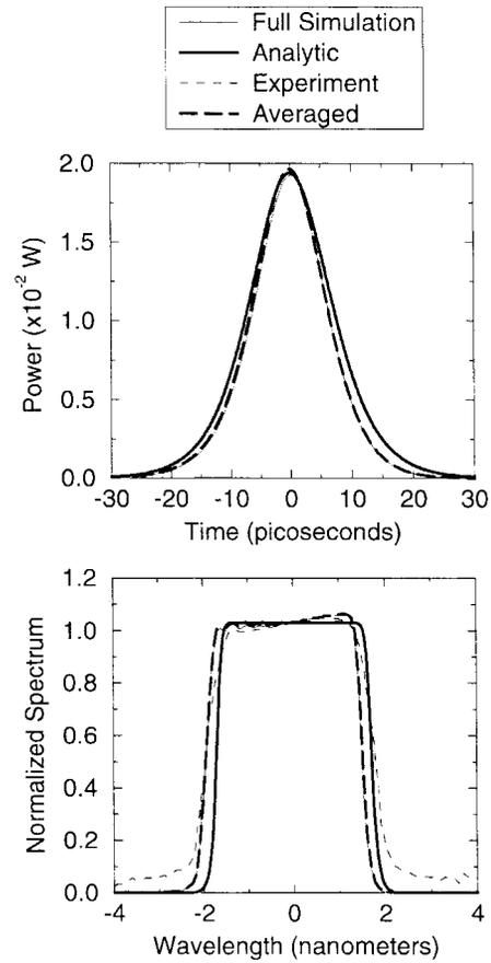
Fig. 8. Steady-state pulse profiles and optical spectra given by (1)–(4) and comparison of this model with the averaged model, the analytic approximation and the experimental findings.
