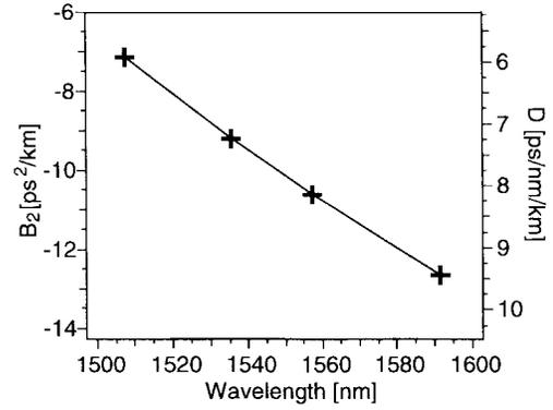
Fig. 14. Measured total dispersion versus wavelength for a typical fiber cavity.
