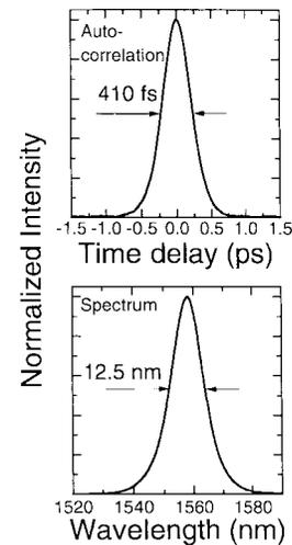
Fig. 2. Typical autocorrelation trace and optical spectrum of the laser output for the anomalous dispersion regime.
