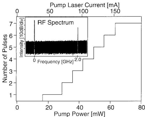
Fig. 11. Number of circulating pulses versus pump power. Inset: RF spectrum of the laser output operating at 2.06 GHz indicating the suppression of lower cavity harmonics by over 30 dB.
