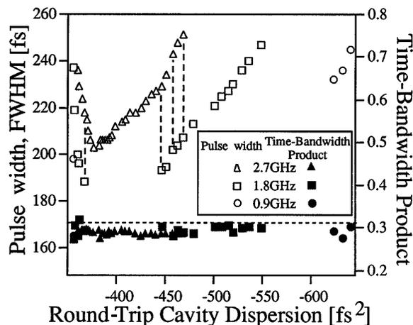
Fig. 3. Pulse width and time-bandwidth product of the mode-locked output with one (circles), two (squares), or three (triangles) pulses circulating in the cavity versus total cavity GVD.
