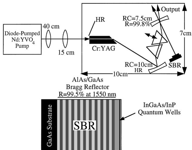
Fig. 1. Diagram of the laser cavity and structure of the SBR. R, reflectivity.
