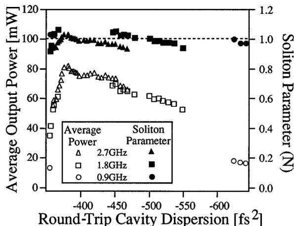
Fig. 4. Total average output power and soliton parameter of the mode-locked output with one (circles), two (squares), or three (triangles) pulses circulating in the cavity versus total cavity GVD.
