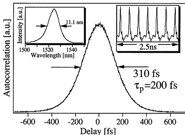
Fig. 2. Autocorrelation and optical spectrum (left inset) of the mode-locked output and a 2.7-GHz pulse train (right inset).
