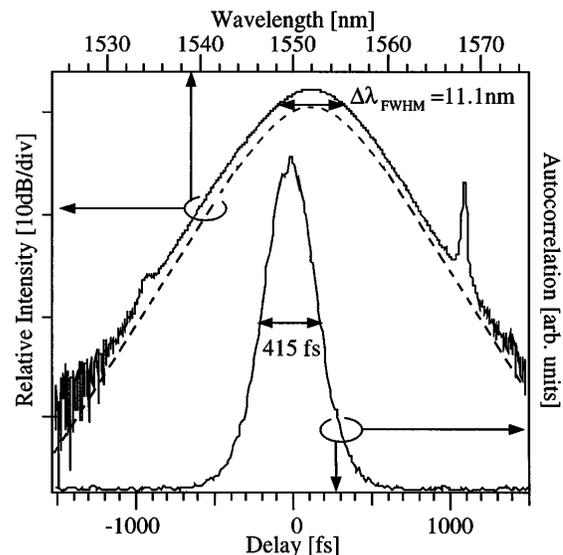
Fig. 2. Typical background-free autocorrelation trace and optical spectrum of the laser output. A  $\text{sech}^2$  curve (dashed) is superimposed.
