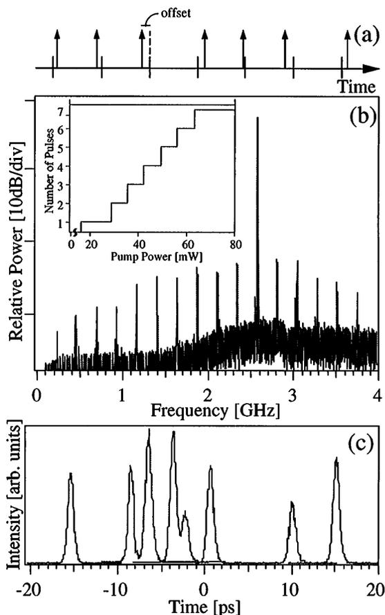
Fig. 3. (a) Example of a pulse train containing temporal offsets between the pulses and their respective locations for an ideally periodic train. (b) rf spectrum of the output with 11 pulses in the cavity. An example of the dependence of the number of circulating pulses on pump power is shown in the inset. (c) Typical cross-correlation trace of adjacent pulses, used to measure directly the periods between adjacent pulses.
