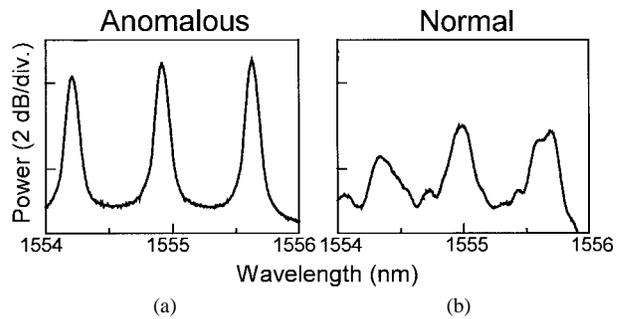
Fig. 8. Comparison of transmitted spectra for (a) anomalous dispersion and (b) normal dispersion chirp fiber in the transmitter. Narrowing is clearly evident in (a) while broadening occurs in (b).
