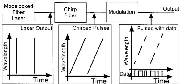
Fig. 1. Schematic of CPWDM transmitter. The wavelength versus time relationship is shown at several points.
