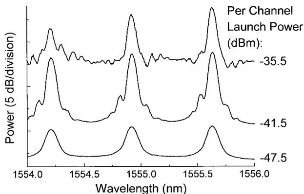
Fig. 7. Transmitted channel spectra for various launch powers showing that the narrowing is clearly power dependent.
