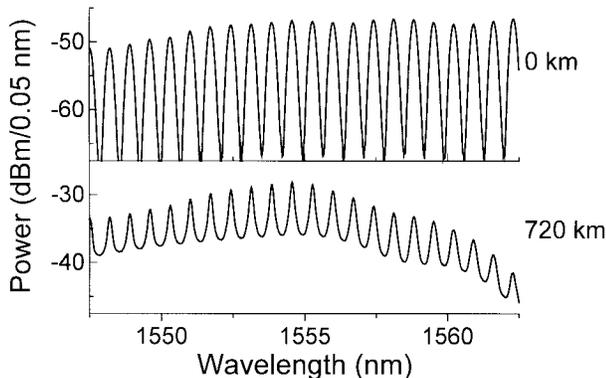
Fig. 6. Measured channel spectra before and after propagation, showing spectral narrowing. The launched power was  $-44$  to  $-46$  dBm per channel, the average power in the transmission line was  $\sim -20$  dBm. The contrast reduction is due to ASE.
