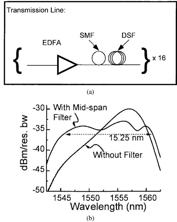
Fig. 4. (a) Schematic of transmission line and (b) the ASE spectrum (with and without gain flattening filter).
