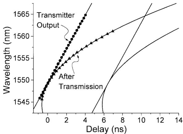
Fig. 5. Time-of-flight measurement of GVD. Dots are measured at output of transmitter, triangles after 720 km propagation. Lines are a parabolic fit to the data. Second set of lines are shifted the time between data pulses to show how dispersion can result in overlap between channels.
