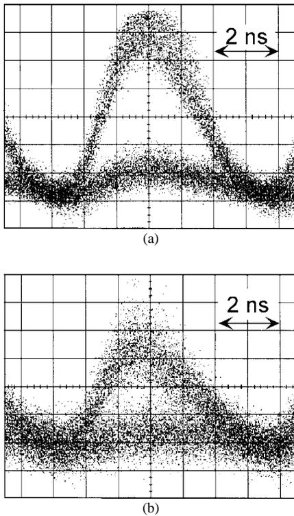
Fig. 10. Eye diagrams after 720 km transmission. For (a), a chirp fiber with anomalous dispersion was used in the transmitter, while for (b), a chirp with normal dispersion was used.
