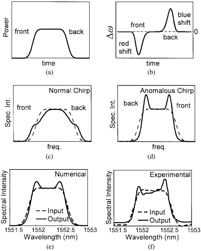
Fig. 9. (a)–(d) Schematic showing how SPM affects a highly chirped, square pulse. (a) Input pulse. (b) The new frequency components generated by SPM. (c) Broadening or (d) narrowing of the spectrum depends on the sign of the initial chirp. In (c) and (d), the dashed line is the initial pulse, solid includes SPM. (e) and (f) Comparison of a numerical calculation including SPM and initial chirp (e) to experimental results (f).
