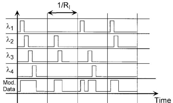
Fig. 2. Time slot diagram of the data for four of the wavelength channels generated by a CPWDM transmitter. The vertical lines denote time slots separated by the time between laser pulses, i.e.,  $1/R_l$  where  $R_l$  is the laser repetition rate. The bottom section shows the data applied to the modulator.
