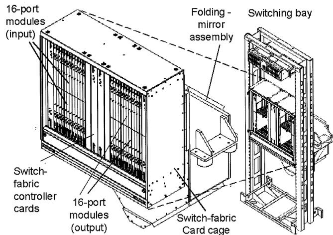
Fig. 2. Mechanical design of modular switch fabric.
