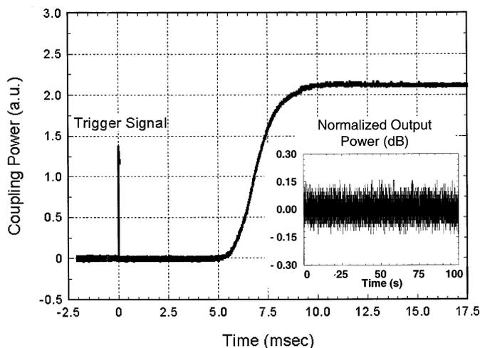
Fig. 3. Typical OXC event. The switching time is measured from the trigger pulse. Inset: fiber-coupled power stability measurement over 100 s.
