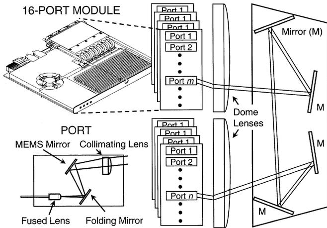
Fig. 1. Schematic of modular optical system.
