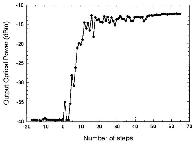
Fig. 4. Typical automatic power-peaking event starting from  $\sim 30$  dB below peak power coupling.
