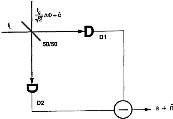
Fig. 5. Schematic of the homodyne detection.
