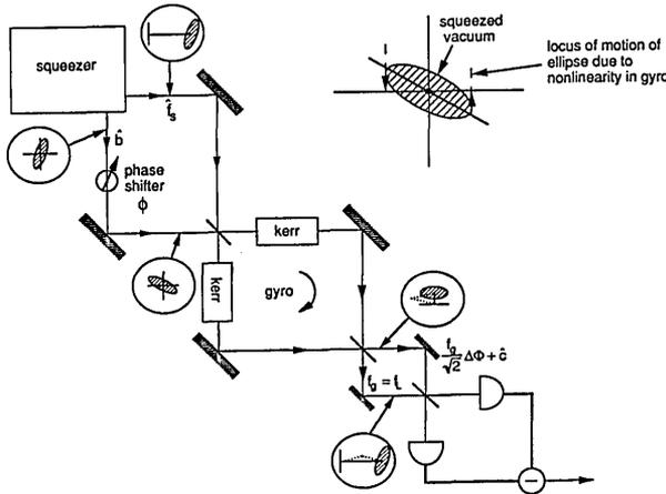
Fig. 4. Squeezer followed by a nonlinear gyro, with squeezed vacuum preparation at input to gyro.
