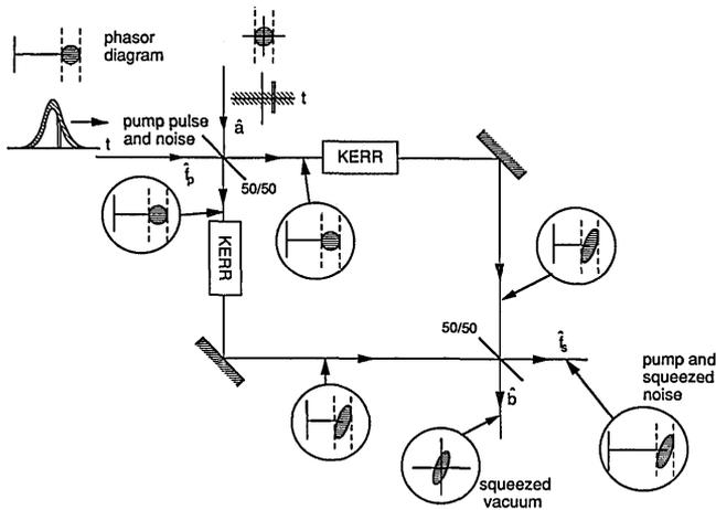
Fig. 2. Equivalent Mach-Zehnder squeezer.
