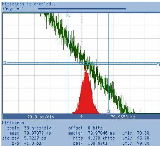
Figure 10. Opto-electronic Transmitter – Jitter Measurements
