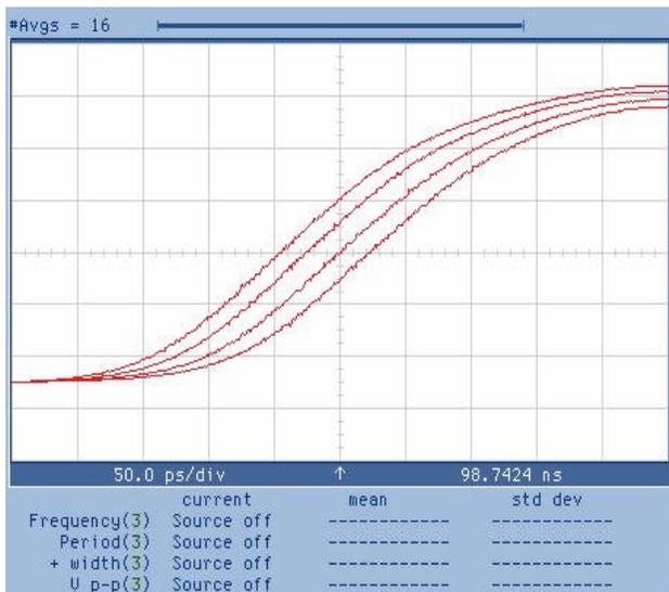
Figure 7. Opto-electronic Transmitter - 20ps Edge Placement Resolution
