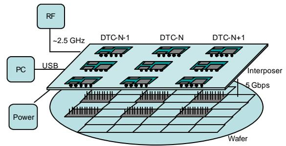
Figure 13. Parallel (array) testing using multiple DTCs.
