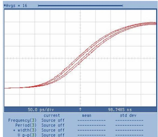
Figure 8. Opto-electronic Transmitter - 10ps Edge Placement Resolution
