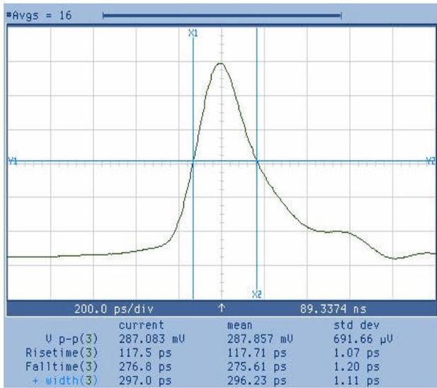
Figure 6. Opto-electronic Transmitter - Minimum Pulse Width
