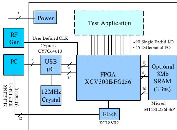
Figure 1. Digital Test Core Block Diagram.
