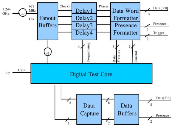
Figure 3. Opto-electronic Tx/Rx Block Diagram.
