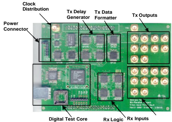
Figure 4. Multi-gigahertz Tx/Rx Photograph [2].
