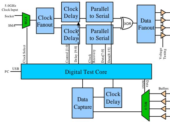
Figure 14. Nano-scale wafer-prober - Block Diagram
