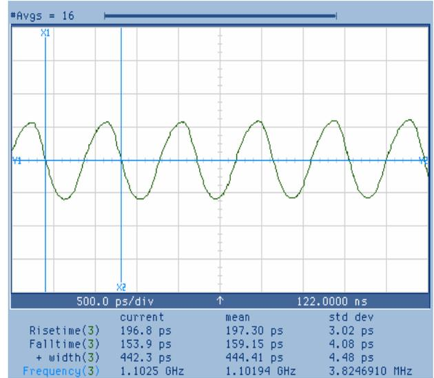
Figure 16. Nano-scale Wafer-prober – Half-speed Signal Output (2.2Gbps)
