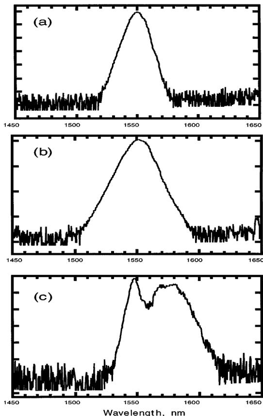
Fig. 3. Input (a) and output pulse spectra of a 182-fs  $N = 1.8$  soliton after propagating through 3.5 m (b) and 9 m (c) of standard PM fiber.
