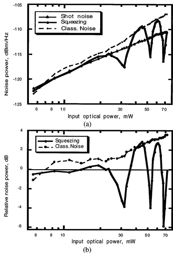
Fig. 2. Absolute (a) and relative (b) noise power fluctuations versus optical power incident into the 88%-reflection port.
