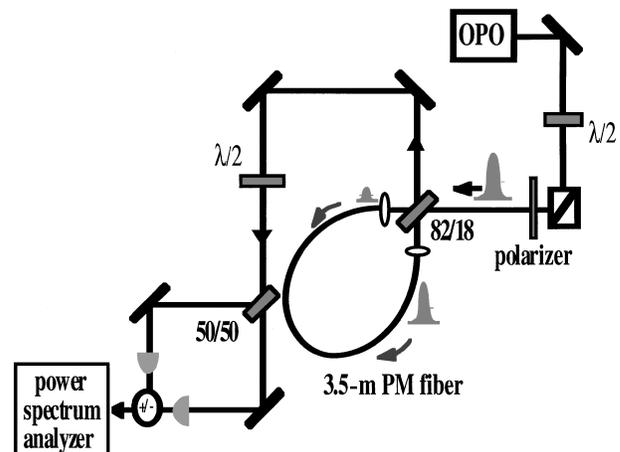
Fig. 1. Experimental setup: OPO, optical parametric oscillator;  $\lambda/2$ , half-wave plates.
