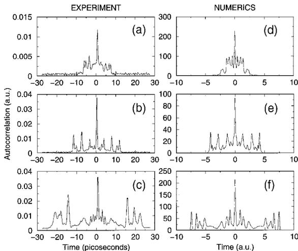
Fig. 3. Left, experimentally achieved autocorrelation as a function of input powers of (a) 9, (b) 13, and (c) 19 mW and, right, autocorrelation generated from the numerical data of Fig. 1 at (d)  $Z = 1$ , (e)  $Z = 2$ , and (f)  $Z = 4$ .
