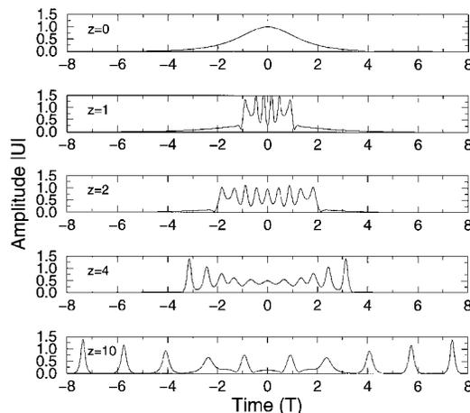
Fig. 1. Numerical simulation of Eq. (1), showing the breakup of a pulse given a strongly chirped initial condition in a low-dispersion, anomalous optical fiber. Note the ejection of pairs of fundamental solitons that propagate away from the center with a speed that is determined by their height.
