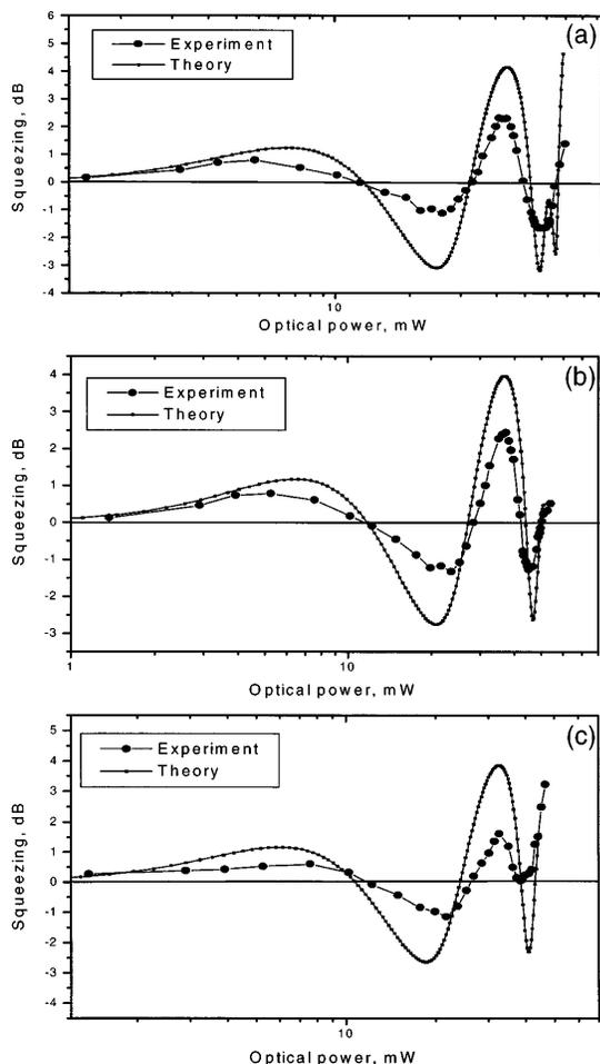
Fig. 3. Numerical simulation plots for a 140-fs pulse propagating through (a) 1.1, (b) 0.875, and (c) 0.580 dispersion lengths in the normal-dispersion regime, with the corresponding experimental plots of squeezing versus input optical power at 1490, 1505, and 1525 nm.
