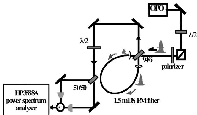
Fig. 1. Experimental setup: OPO, optical parametric oscillator;  $\lambda/2$ 's, half-wave plates; DS PM, dispersion-shifted polarization-maintaining.
