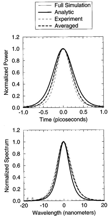
Fig. 9. Comparison of the experimental autocorrelation measurements (scaled with the assumption that the pulse shape is a hyperbolic secant) and output spectrum with the full evolution equations [Eqs. (1), (4), and (11)], the averaged equation [Eq. (13)], and the approximate analytic solution with no slow response [Eqs. (14)–(19)].
