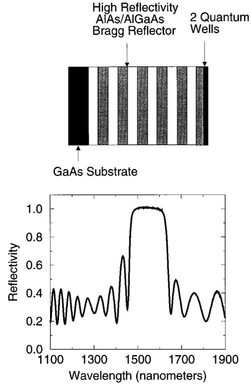
Fig. 2. SBR structure and its associated reflectivity spectrum.
