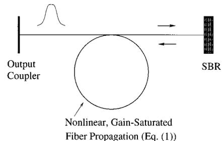
Fig. 1. Schematic of mode-locking fiber laser, which includes a 1% output coupler, SBR, and a gain-saturated fiber segment.
