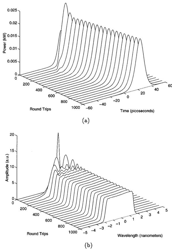
Fig. 6. Numerical simulation of the pulse evolution as governed by Eqs. (1), (4), and (11) in both (a) the time and (b) the frequency domain for a fiber cavity with an average normal dispersion value of  $\bar{D} = -38.1$  ps/(km nm). In (a) the pulse is seen to mode lock to a  $\sim 13.6$  ps chirped pulse whose spectral evolution is given by (b).
