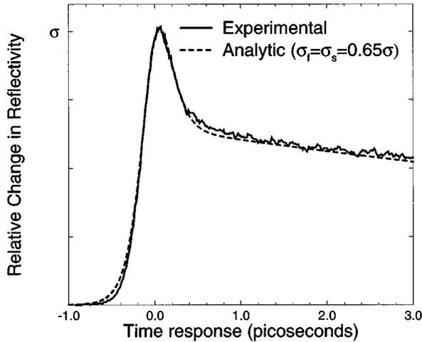
Fig. 4. Comparison of the experimental pump and probe measurements of the SBR at  $1.55 \mu\text{m}$  with the jump condition of Eq. (7), which includes a fast response and slow saturation response with relaxation. Here, an  $\sim 400$ -fs hyperbolic-secant pulse is assumed for  $Q_-$ , and  $\sigma_f = \sigma_s = 0.65\sigma$  with  $T_d = 14$ .
