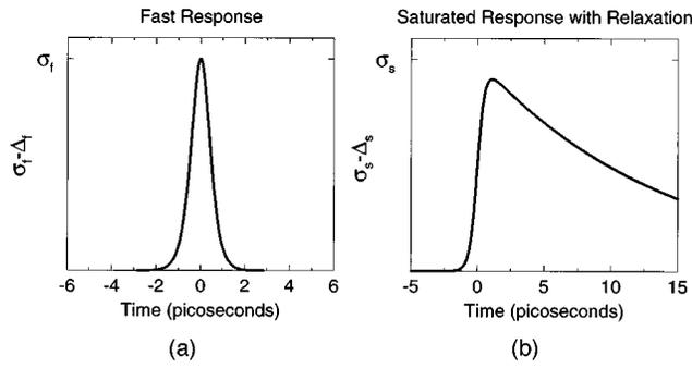
Fig. 3. (a) Change in reflectivity  $\sigma_f - \Delta_f$  corresponding to the fast response. (b)  $\sigma_s - \Delta_s$  gives the change in reflectivity that is due to the slow saturated response with relaxation. Note that  $Q_-$  corresponds to a 1-ps hyperbolic-secant pulse.
