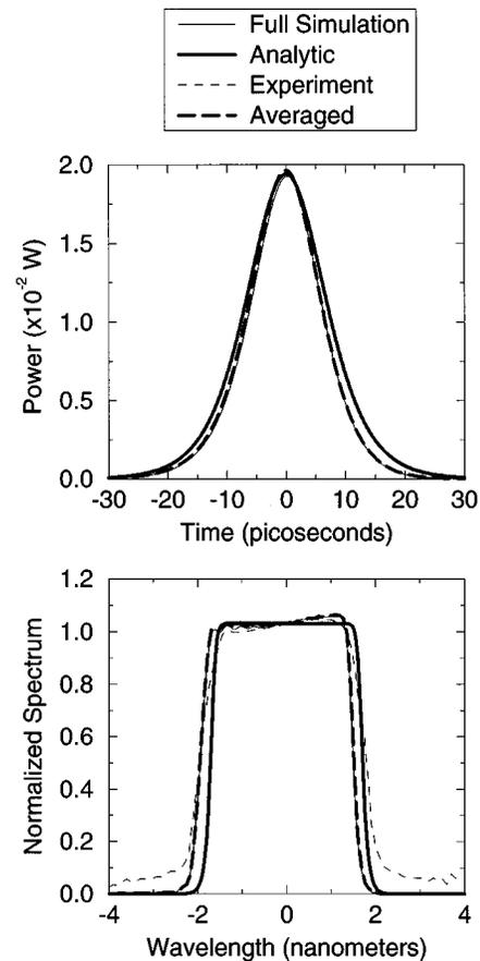
Fig. 7. Comparison of the experimental results with  $\bar{D} \approx -38$  ps/(km nm) and the full evolution equations [Eqs. (1), (4), and (11)], the averaged equation [Eq. (13)], and the approximate solution with no slow response [Eqs. (14)–(19)]. Note the remarkable agreement between all three models and the experimental results. The 13.5-ps pulse width is consistent with experimental observation.
