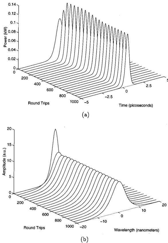
Fig. 8. Numerical simulation of the pulse evolution as governed by Eqs. (1), (4), and (11) in both (a) the time and (b) the frequency domain for a fiber cavity with an average anomalous dispersion value of  $\bar{D} \approx 12$  ps/(km nm). In (a) the laser is seen to mode lock to an  $\sim 420$ -fs chirped pulse with a time-bandwidth product of  $\sim 0.4$  and whose spectral evolution is given by (b).
