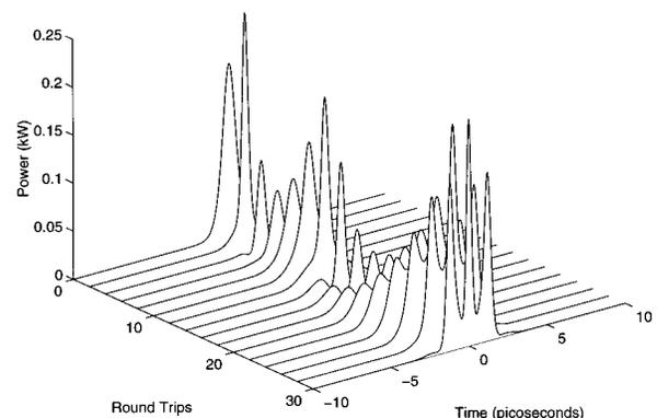
Fig. 10. Typical evolution of a pulse governed by full evolution equations (1), (4), and (11) in the anomalous dispersion regime  $\bar{D} \approx 12$  ps/(km nm). Note that for the estimated experimental parameter values the pulse begins to break up into a group of multiple pulses. In this simulation we have taken  $\sigma_s = 0$  and  $\sigma_f = 2.6\%$ .
