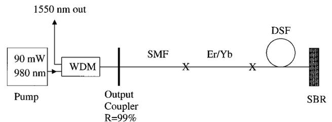
Fig. 5. Experimental setup of mode-locking laser cavity with a 1% output coupler, SBR, and average dispersion in the anomalous regime. The 980-nm pump is coupled through a wave-length division multiplexer (WDM) into the laser cavity, which consists of three fiber segments: a single-mode fiber (SMF), an erbium–ytterbium fiber (Er/Yb), and finally a dispersion-shifted fiber (DSF).
