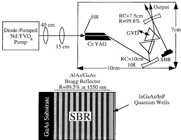
Fig. 4. Schematic of the  $\text{Cr}^{4+}$ :YAG laser cavity and structure of the SBR. (HR: high reflector; RC: radius of curvature; R: reflectivity).
