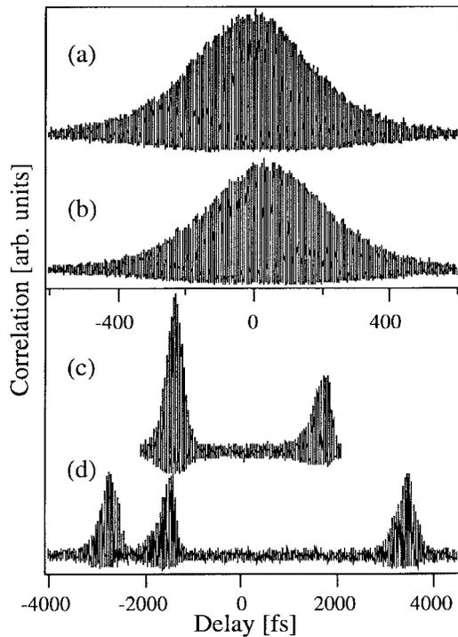
Fig. 6. (a) Autocorrelation and (b)–(d) cross correlations of the  $\text{Cr}^{4+}$ :YAG laser with three pulses in the cavity. The pulses are equally spaced in (b) and not equally spaced in (c) and (d).
