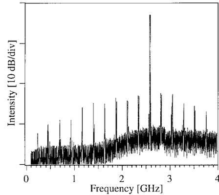
Fig. 8. RF spectrum of the Er–Yb laser output operating with 11 pulses in the cavity.
