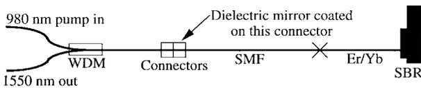
Fig. 7. Schematic of the Er–Yb fiber laser. WDM: wavelength division multiplexer; SMF: single-mode fiber.
