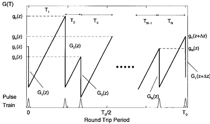
Fig. 3. Qualitative depiction of the time-dependent gain with  $N$  pulses in the cavity.
