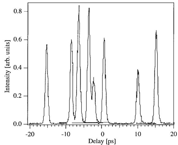
Fig. 9. Cross correlation of the Er–Yb laser output operating with 11 unequally spaced pulses in the cavity.
