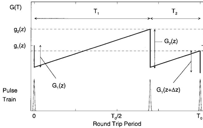
Fig. 2. Qualitative depiction of the time dependent gain with two pulses in the cavity.
