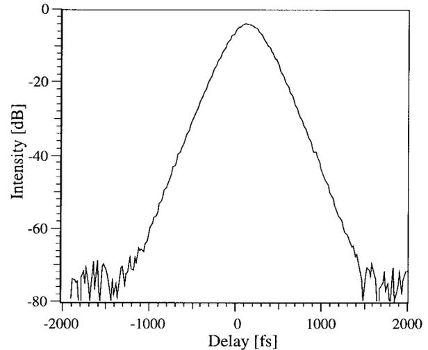
Fig. 10. Plot of the log of the pulse autocorrelation of the  $\text{Cr}^{4+}$ :YAG laser showing the absence of any continuum to  $\approx 40$  dB.
