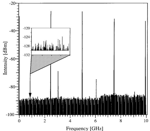
Fig. 5. RF spectrum of the  $\text{Cr}^{4+}$ :YAG laser output operating with three pulses in the cavity. The inset shows a 4-kHz span with a 1-Hz resolution bandwidth centered about the cavity fundamental frequency illustrating that this component is suppressed by over 110 dB from the harmonic frequency around 2.5 GHz. The tones at 3, 6, and 9 GHz are believed to originate from pump light.
