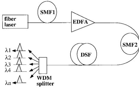
Fig. 1. Experimental setup for spectral broadening. SMF is single mode fiber, DSF is dispersion shifted fiber, EDFA is Er-doped fiber amplifier.
