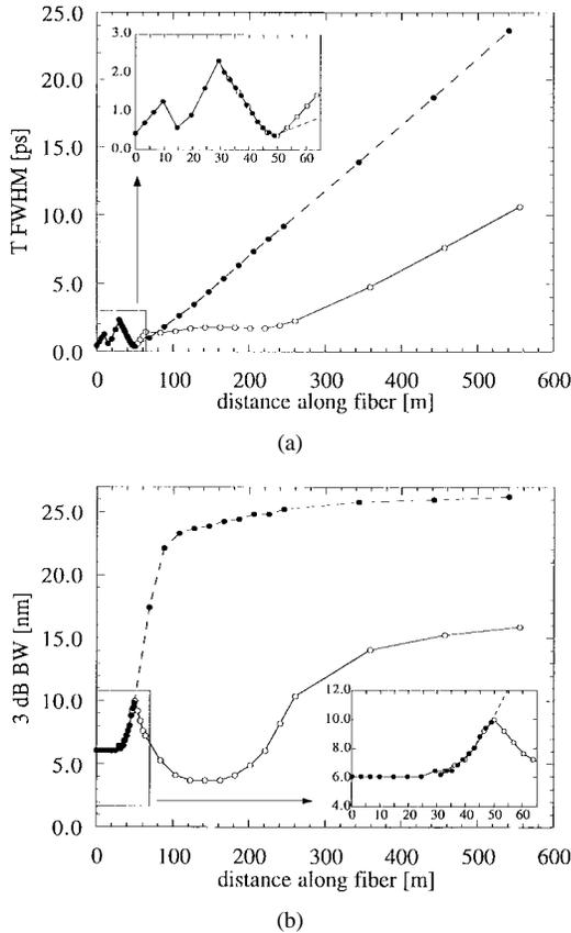
Fig. 2. Numerical simulation results of the evolution of the (a) temporal and (b) spectral widths of the pulse as a function of propagation distance in the fiber section for the cases of SMF2 = 35 m (open circles, solid lines) SMF2 = 20 m (filled circles, dashed lines). The insets show the evolutions in the first three fiber sections: SMF1, EDFA, and SMF2.
