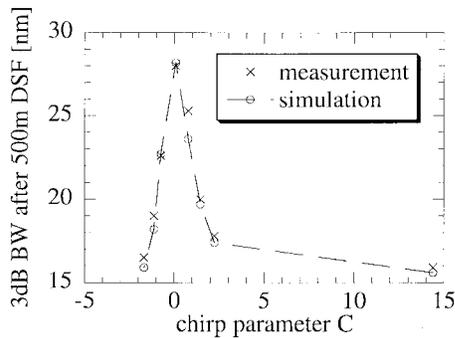
Fig. 4. Final 3-dB spectral bandwidth as a function of the pulse chirp parameter entering the DSF. Experimental values of the chirp parameter (shown by  $\times$ ) were estimated from the measured pulse time-bandwidth product. Chirp parameters obtained from simulation results are shown with circles. The largest chirp corresponds to no SMF2. Adding SMF2 decreases the chirp, with the smallest value of chirp corresponding to 35 m of SMF2.
