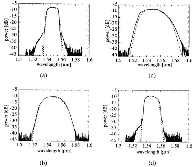
Fig. 3. Final measured spectra for (a) positively prechirped case, (b) nearly transform limited case, and (d) negatively prechirped case. The broadest spectrum achieved with the laser operated at 2.5 GHz is shown in (c). The solid lines correspond to the experimental data, and the dashed lines to the numerical results.
