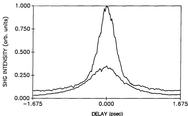
Fig. 2. Signal pulse at output: polarizer parallel to signal, orthogonal to control. Lower trace: orthogonal control pulse absent—no solitary wave collisions. Upper trace: control pulse present—enhanced transmission through solitary wave collisions. SHG, second-harmonic generation.
