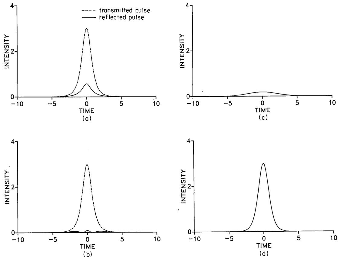
Fig. 4. Transmitted and reflected intensity profiles for normalized input energies of 3.5, 3.0, and 0.5 shown in plots (a), (b), and (c), respectively. The input pulse is shown for comparison (d).
