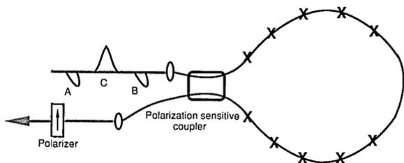
Fig. 9. Alternative XOR gate configuration. Note that both the signal and control pulses enter through the same input port.
