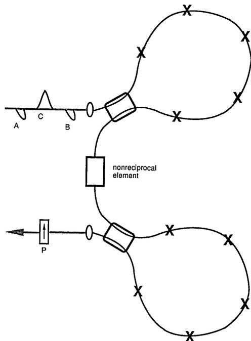
Fig. 10. Proposed regenerative AND gate with fan-out, utilizing solitary-wave collisions. Two loops (cf. Fig. 5) are in series, with a nonreciprocal element between the loops. A and B are the incoming pulses, while C is a locally generated higher-intensity pulse.
