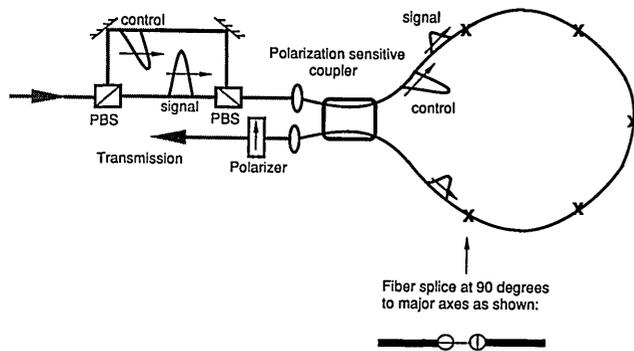
Fig. 5. Proposed simple ring interferometer AND gate employing solitary-wave collisions with birefringent fiber sections (six sections shown). This device can be used as a pulse regenerator. The X's indicate fiber splices. PBS, polarizing beam splitter.
