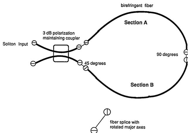
Fig. 2. Proposed fiber loop intensity switch with rotated birefringence axes.
