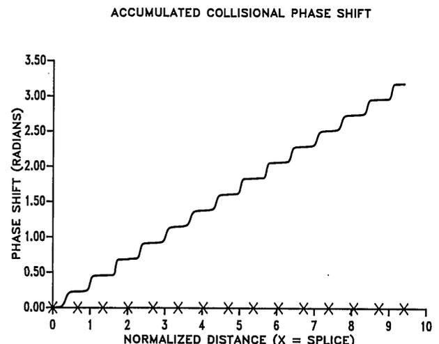
Fig. 6. Phase shift of one pulse, accumulated through 14 solitary-wave collisions, as a function of distance. The phase is in radians. The X's indicate fiber splice locations.
