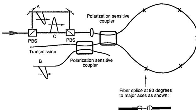
Fig. 8. Simple ring interferometer XOR gate configuration. The gate is regenerative and has fan-out.
