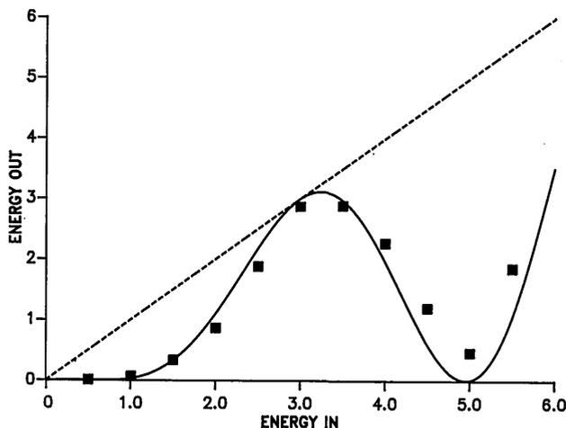
Fig. 3. Output pulse energy versus input pulse energy. The curve is computed from Eqs. (2) and (3). The points are computed from simulations.
