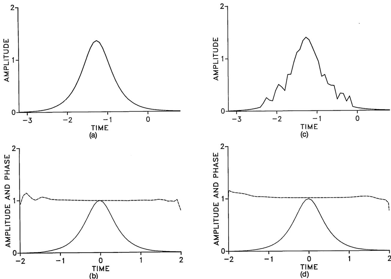
Fig. 7. Predicted pulse profiles after traversing a 14-section loop: (a) control (at input), (b) half-signal after 14 collisions. Plots (c) and (d) are the same as (a) and (b) but with noisy, degraded control. The solid curve is the amplitude. The dotted curve is the collision-induced phase in units of  $\pi$  radians.
