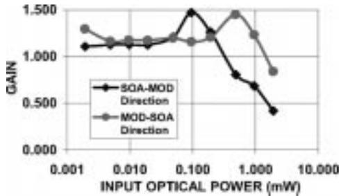
Fig. 2. Directional dependence of gain versus input optical power at 100-mA SOA drive current. Gain is expressed as a linear ratio. The laser is operated with intracavity powers where the gain is maximized.
