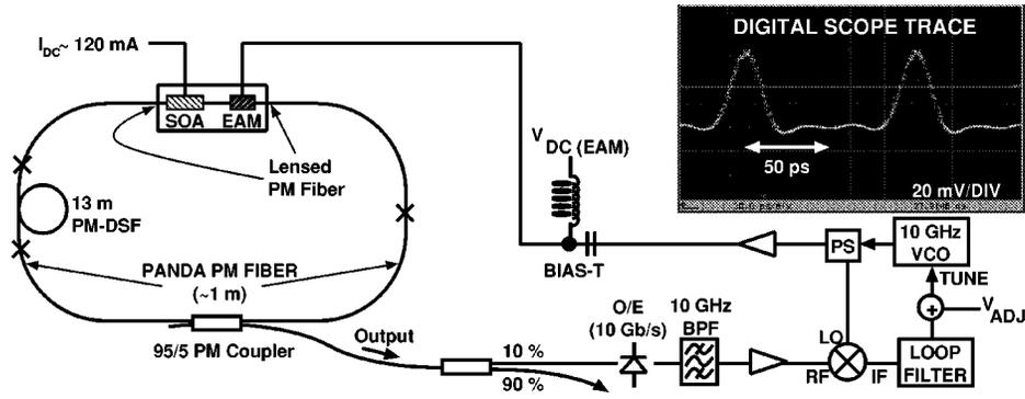
Fig. 1. Mode-locked laser schematic with digital sampling scope trace of pulsetrain.
