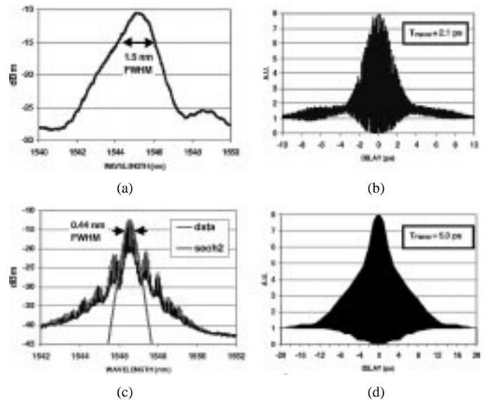
Fig. 3. (a) and (b): Optical spectrum and autocorrelation trace, respectively, for  $\bar{D} = +7.0$  ps/nm/km. (c) and (d):  $\bar{D} = +0.8$  ps/nm/km.
