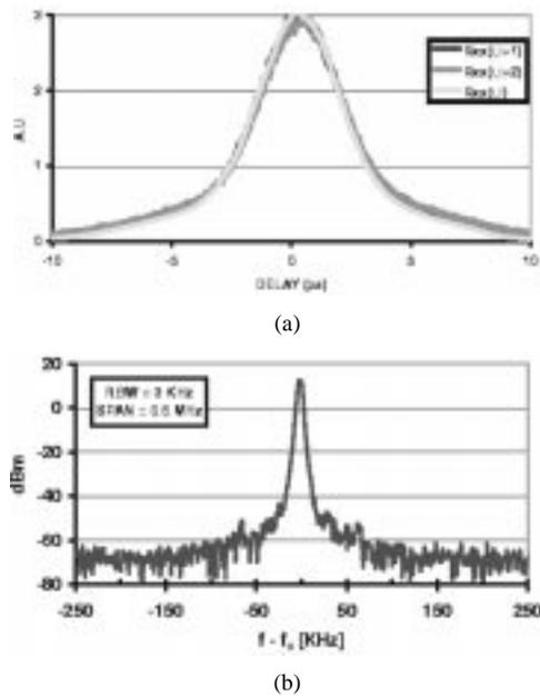
Fig. 4. (a): Noninterferometric autocorrelation ( $R_{xx}(i, i)$ ), first-order cross correlation ( $R_{xx}(i, i + 1)$ ), and second-order cross correlation ( $R_{xx}(i, i + 2)$ ) showing  $< 100$  fs timing jitter. (b): RF spectrum of 10-GHz laser mode.
