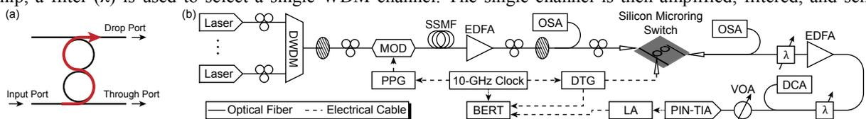
Fig. 2. (a) Second-order micro-ring resonator. Arrow indicates the optical path for the drop port. (b) Diagram of the experimental setup.
