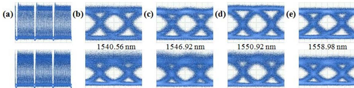
Fig. 2: Input (top) and output (bottom) of (a) the optical packets; (b)-(e) 40-Gb/s eye diagrams of a subset of payload wavelength channels.
