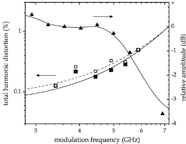
Fig. 5. Amplitude Bode plot and THD measurements plotted against the sinusoidal modulation frequency for the highest wavelength signal. The amplitude measurements ( $\blacktriangle$ ) were taken while modulating a single ring. The THD measurements, shown with exponential curve fits, were taken while modulating both a single ring ( $\blacksquare$ ) and four simultaneous rings ( $\circ$ ).
