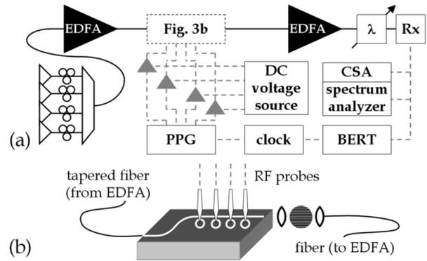
Fig. 3. (a) Experimental measurement and (b) chip-coupling setups. Lasers (open triangles), multiplexer (trapezoid), polarizer (circle), grating filter ( $\lambda$ ), receiver (Rx), electrical amplifiers and bias tees (gray triangles), optical fiber (solid lines), and coaxial cable (dashed lines) are among the components.
