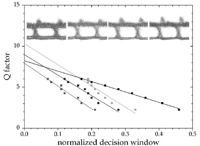
Fig. 4.  $Q$ -factor extrapolations from time-window measurements for the four modulated signals. The measured  $Q$ -factor (■) is plotted against the fraction of the eye sampling window with linear curve fits. The curves appear from lowest (darkest) to highest wavelength (lightest). Eye diagrams for the four optical signals are given from lowest (left) to highest (right) wavelength.
