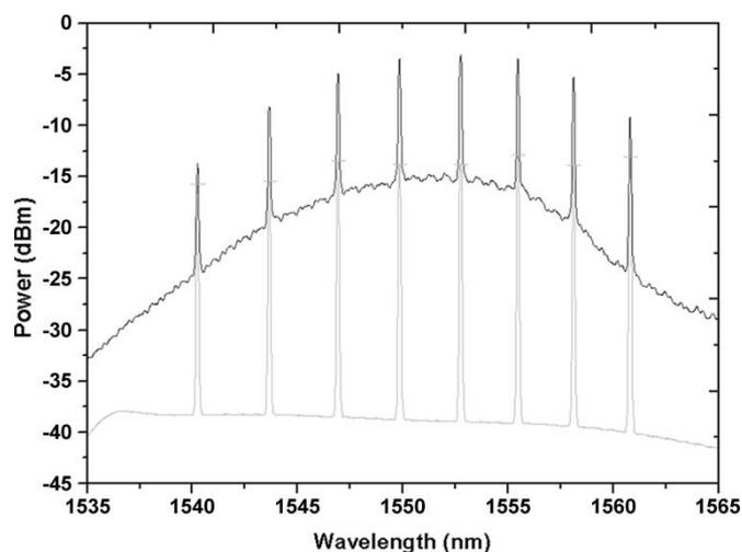
Fig. 8. Multichannel spectrum profile: the input packet spectrum (light gray) and after 58 node hops (dark gray) defined as the average power, taking into account the 0.67% duty cycle where one 25.6-ns-long packet is sent through the recirculating loop every 3.84  $\mu$ s.
