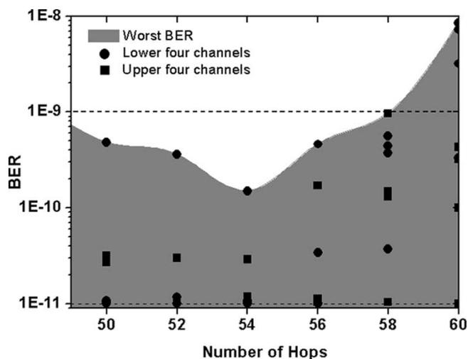
Fig. 7. BER for eight payload channels versus number of hops; dashed line for BER of  $10^{-9}$ . The BER measurement of each payload channel falls within the gray region. Annotation of the spectrum parameters emphasized in the phenomenological model.
