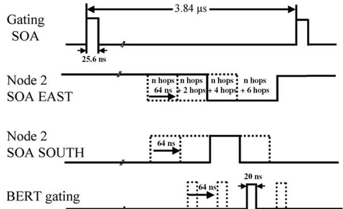
Fig. 5. Packet synchronization. The SOA control signals and the gating signals are delayed by 64 ns to increment the propagation by one loop. One loop consists of two hops. SOA SOUTH is switched ON to drop the packet for BER measurement while SOA EAST is switching OFF.
