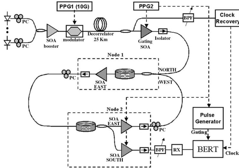
Fig. 4. Experimental setup of the switching-loop test-bed (PPG1: fast programmable pattern generator; PPG2: slow programmable pattern generator; PC: polarization controller; SOA: semiconductor optical amplifier; boxed arrow: optical isolator; BPF: bandpass filter; MOD: LiNbO<sub>3</sub> modulator; RX: optical receiver module; BERT: BER tester).
