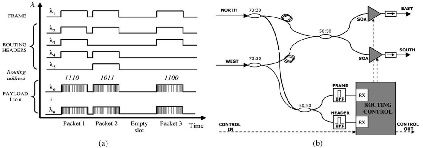
Fig. 2. (a) Packet structure: payload and routing headers encoded on DWDM channels. (b) Switching node configuration of the data vortex network (BPF: optical bandpass filter; RX: optical receiver module; plain line: optical signal; dashed line: electrical signal).
