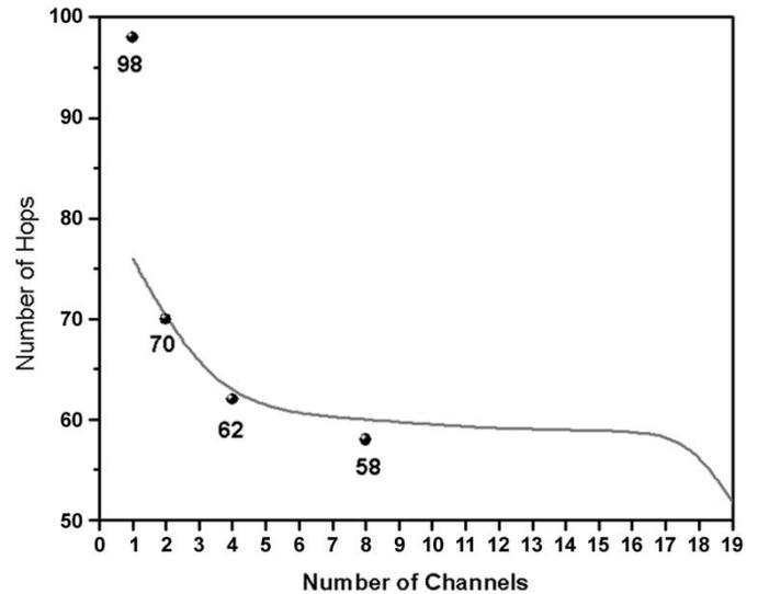
Fig. 11. Experimental results for one, two, four, and eight channels. The maximum number of hops is set for bit error measurement below  $10^{-9}$  for all WDM channels. The solid gray line shows simulation results. Functional bandwidth for eight payload channels versus number of hops. The solid gray line represents the simulation results.
