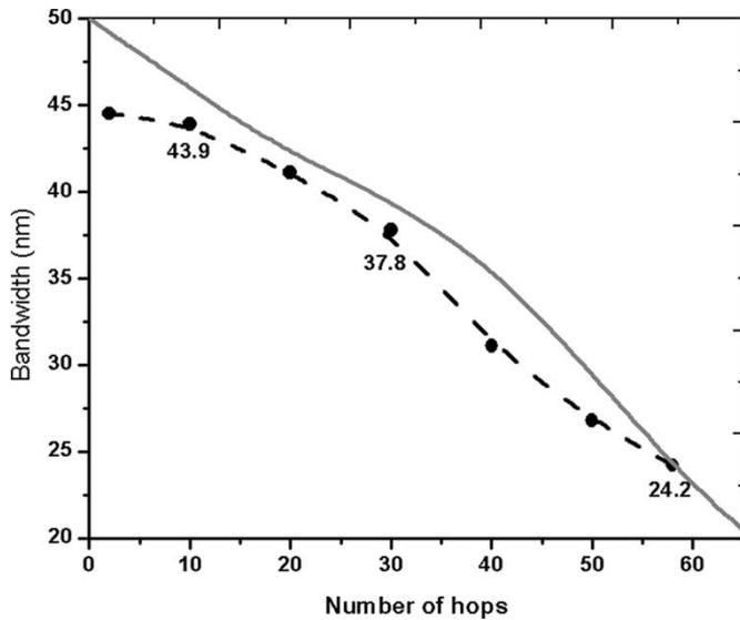
Fig. 10. Functional bandwidth for eight payload channels versus number of hops. The solid gray line represents the simulation results.
