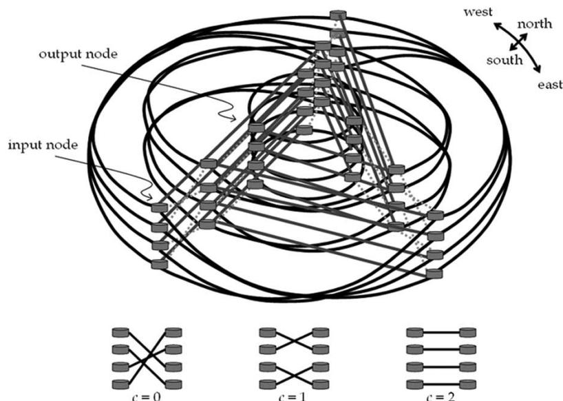
Fig. 1. Data vortex topology with  $A = 3$ ,  $H = 4$ ,  $C = 3$  corresponding to a 12-port interconnection network that contains 36 switching nodes.
