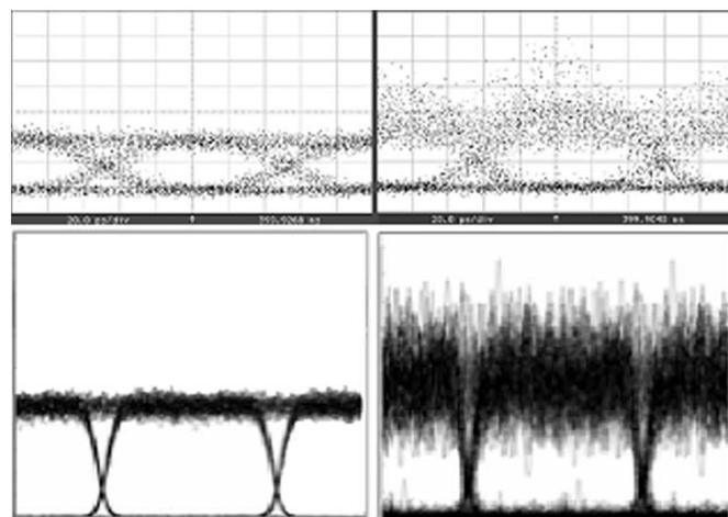
Fig. 9. Optical eye diagram of channel at 1558.10 nm after 2 and 58 hops. Simulated eye diagram of one channel after two hops (left) and after 58 hops (right).
