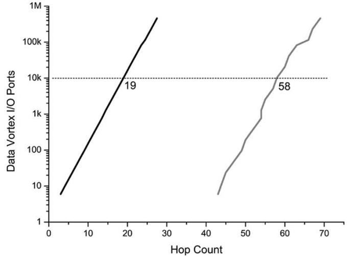
Fig. 3. Data vortex I/O port size versus hop count under heavy load. Network size for the median number of hops (black) and for the 99.999th percentile of the injected packets (gray).
