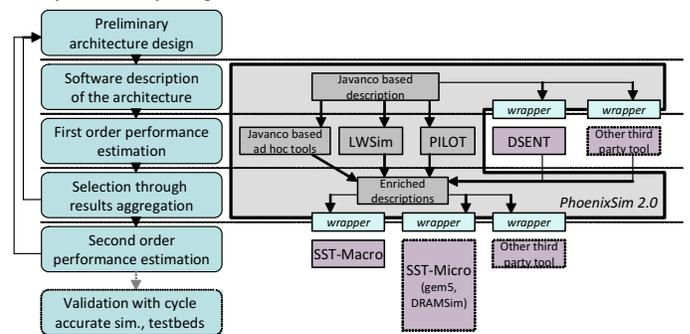
Figure 1. Figure 1: Schematics of our targeted design flow
