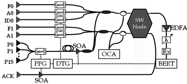
Fig. 3. Optical testbed, designed to construct and analyze the wavelength-parallel messages and *ack* pulses. (PPG: pulse pattern generator. DTG: data timing generator. OCA: optical communications analyzer.)
