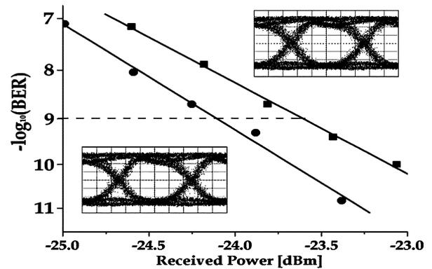
Fig. 5. BER curves and eye diagrams are given for back-to-back ( $\bullet$ , left eye) and node output ( $\blacksquare$ , right eye). The power penalty of the node is measured to be less than 0.5 dB at BER =  $10^{-9}$  ( $\lambda = 1554.42$  nm).
