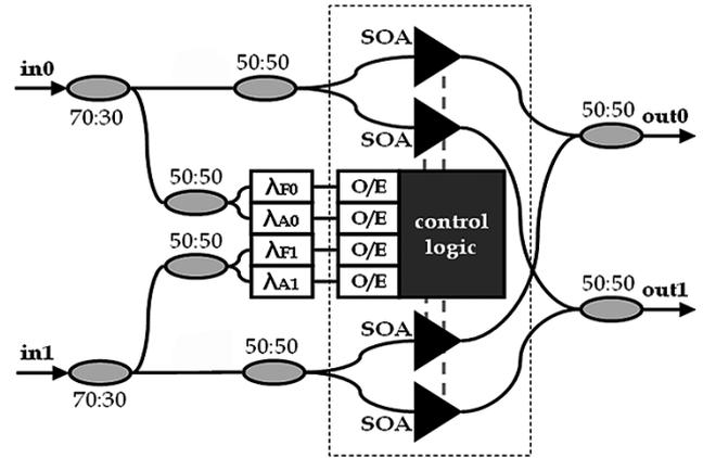
Fig. 2. Experimental node is comprised of SOAs, optical couplers (ellipses, with coupling ratios), wavelength filters ( $\lambda$ ), p-i-n receivers (O/E), optical fibers, and an electronic control circuit implemented by a CPLD.
