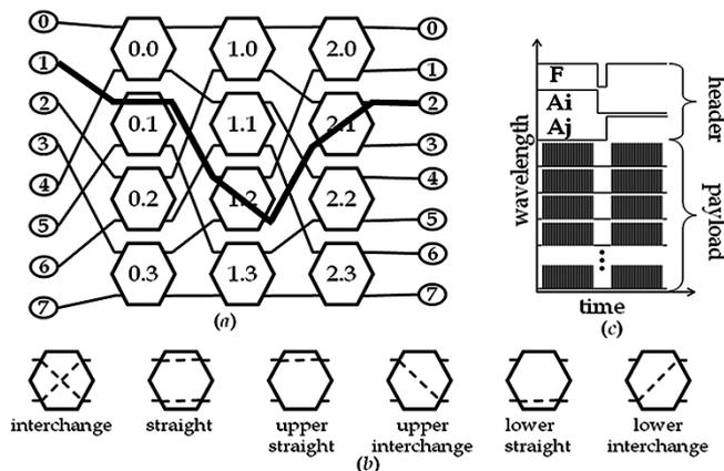
Fig. 1. (a) Omega network with a lightpath across it. (b) Each node has six switching states. (c) The wavelength parallel messages.
