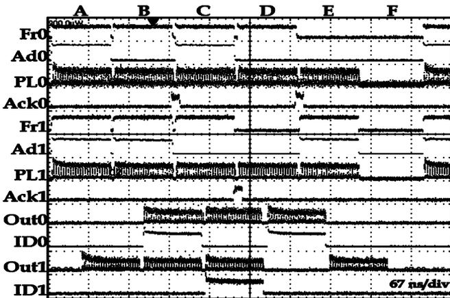
Fig. 4. Optical signals at the inputs (per input: frame, address, payload, and *ack*) and the outputs (per output: payload and source id) demonstrate the correct routing functionality and reception of *acks* over six slots (A through F). *Acks* are generated only in output Port 0. Four messages are sent from each input port (the same payload is driven to both ports, but the frame qualifies only four messages per port).
