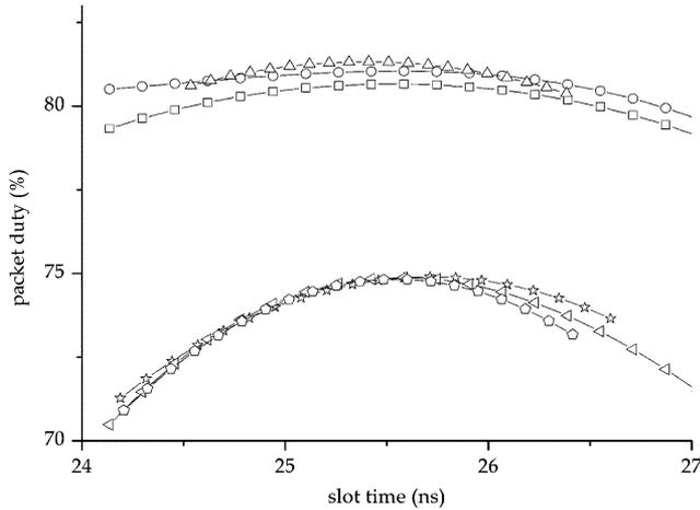
Fig. 4. Plot of the maximum packet duty versus slot time for the given six-packet sequence, with curves showing the manifestation of a generally parabolic relationship near the optimal slot time. The first three packets (#1  $\square$ , #2  $\circ$ , #3  $\triangle$ ) are longer than the last three (deflected) packets (#4  $\triangleleft$ , #5  $\star$ , #6  $\diamond$ ).
