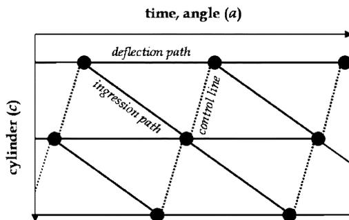
Fig. 1. Graphical representation of the data vortex deflection signal timing requirement, in which packets propagate from node ( $\bullet$ ) to node on fiber-optic paths (—). Ingression path latencies must be shorter than deflection path latencies in order to allow time for deflection signals to be sent on control lines (---).
