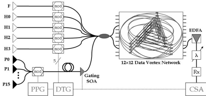
Fig. 2. Schematic of experimental setup with the appropriate packet generation and detection subsystems containing five routing header wavelengths ( $F$  and  $H0$  through  $H3$ ) and 16 payload wavelengths ( $P0$  through  $P15$ ), with  $\text{LiNbO}_3$  modulators (mod), pulse pattern generator (PPG), data timing generator (DTG), communications signal analyzer (CSA), erbium-doped fiber amplifier (EDFA), tunable filter ( $\lambda$ ), and high-speed dc-coupled postamplified receiver (Rx).
