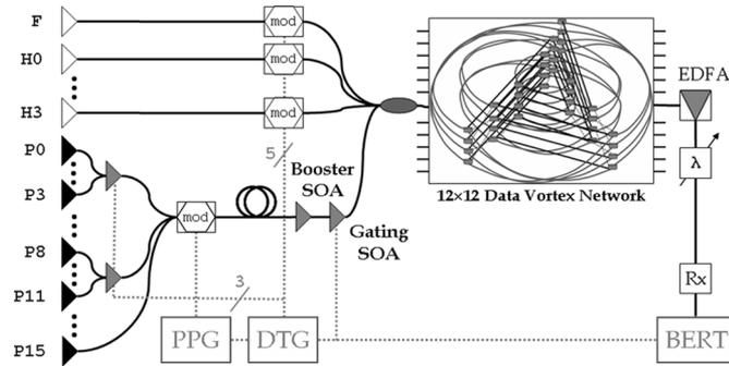
Fig. 2. Schematic of experimental setup with the appropriate packet generation and detection subsystems, with  $\text{LiNbO}_3$  modulators (mod), pulse pattern generator (PPG), data timing generator (DTG), BER tester (BERT), EDFA amplifier, tunable filter ( $\lambda$ ), and high-speed receiver (Rx). The payloads are grouped into four sets of four in order to produce packets with a variable number of wavelengths.
