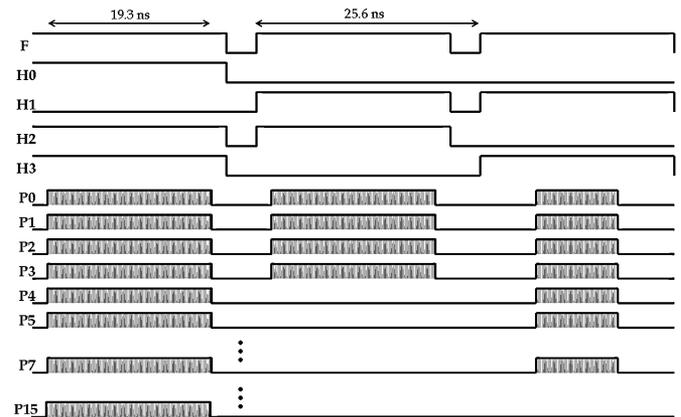
Fig. 1. Illustration of different possible payload formats for the multiple-wavelength packet. The first contains all 16 payload wavelengths with a duration of 19.3 ns; the second, four wavelengths and 19.3 ns; the third, eight wavelengths and 9.6-ns offset to the center of the timeslot.
