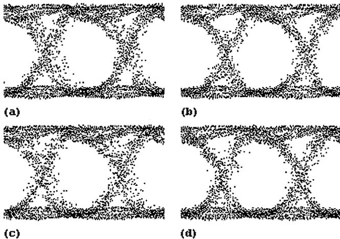
Fig. 5. Eye diagrams of output payloads for packet payloads with (a) 4, (b) 8, (c) 12, and (d) 16 wavelengths. The number of wavelengths present in a payload has a greater effect on signal integrity than the payload timing.
