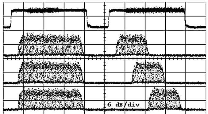
Fig. 4. Waveforms of optical headers and payloads. The first line shows the frame and header wavelengths, which delineate the packet. Subsequent lines illustrate various payload durations and offsets. The packets shown contain a variety of wavelengths, ranging from 4 to 16.
