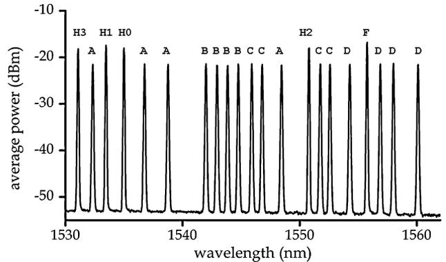
Fig. 3. Plot of packet optical power spectrum, with the five routing header wavelengths higher than the 16 payload wavelengths, which are divided into four groups (A, B, C, D).
