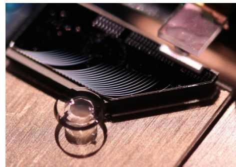
Figure 6: A high-Q MgF2 WGM resonator coupled with a low loss SiN waveguide.
