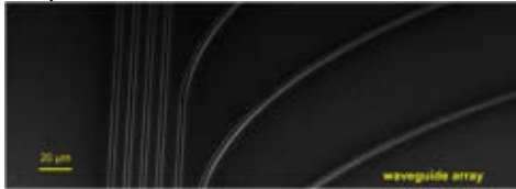
Fig. 5. SEM images showing key components of a MWIR PIC spectrometer fabricated in silicon include a combiner and an array of rib waveguides.
