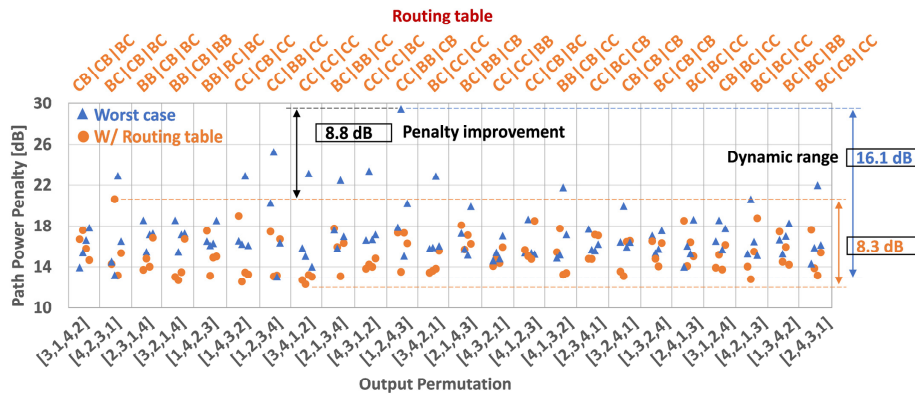
Fig. 5. Detailed port-to-port power penalty of both selected and worst-case path mapping for all 24 permutations. Note that 11 dB of power penalty contributed from in/out grating couplers. Reprinted from [68]
