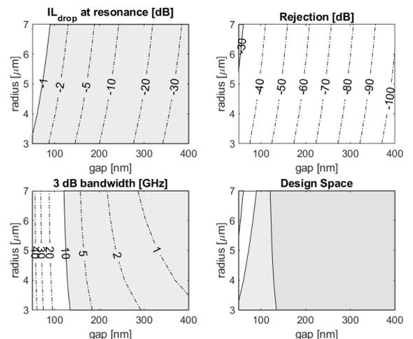
Figure 5. Performance contours and design space of MRR with identical bus widths at 1310 nm.  $w_{bus} = 450$  nm,  $w_{ring} = 450$  nm,  $h_{wg} = 300$  nm,  $h_{slab} = 50$  nm. The white area is the desired design space. (a) IL at resonance. (b) Rejection. (c) Bandwidth. (d) The design space considering all three performance parameters.
