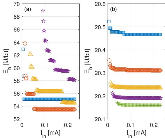
Figure 11. Energy consumption per bit versus TIA input current for data rates of 10 Gbps (rectangular), 15 Gbps (circle), 20 Gbps (triangle), 25 Gbps (pentagram), and 30 Gbps (crossbar). (a) 65 nm platform. (b) 28 nm platform.
