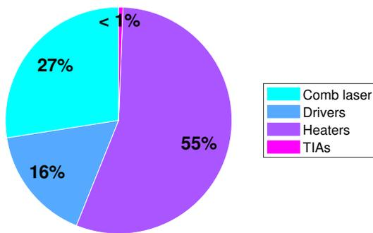
Figure 13. The relative share of overall energy consumption of each component in the analyzed link for data rates of 22 Gbps and 27.5 Gbps.
