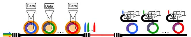
Figure 1. A block diagram of unidirectional SiP DWDM interconnect.
