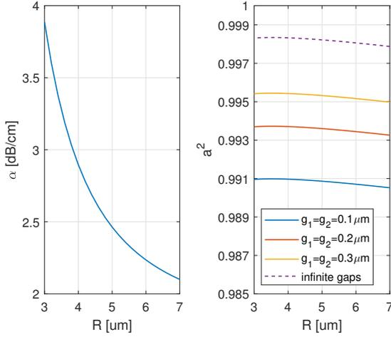
Figure 3. (a) The bending loss of a bent ridge waveguide as a function of radii at 1310 nm. The ridge waveguide parameters are  $w_{wg} = 450$  nm,  $h_{wg} = 300$  nm,  $h_{slab} = 50$  nm. (b) The MRR round-trip power loss as function of radius. Each curve represents a different gap, where  $g_1 = g_2$ .
