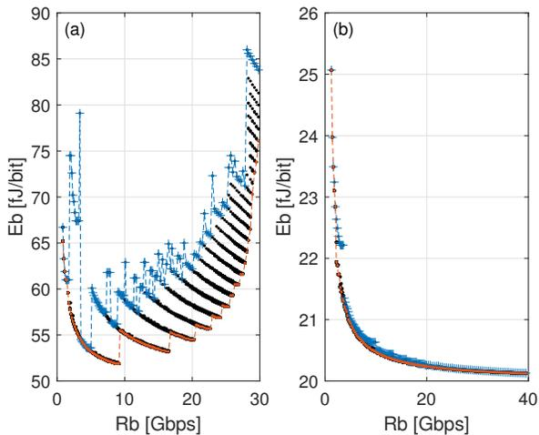
Figure 12. Energy consumption per bit versus data rate. (a) 65 nm platform. (b) 28 nm platform. Each of the dots represents a different TIA input current, and the crossbar marker stands for the energy consumption at  $I_{\text{TIA},\min}(R_b)$ . The Pareto front of the minimum  $E_b$  is marked by the red dots. It can be observed that at  $I_{\text{TIA},\min}(R_b)$ , the power consumption is higher than the Pareto front.
