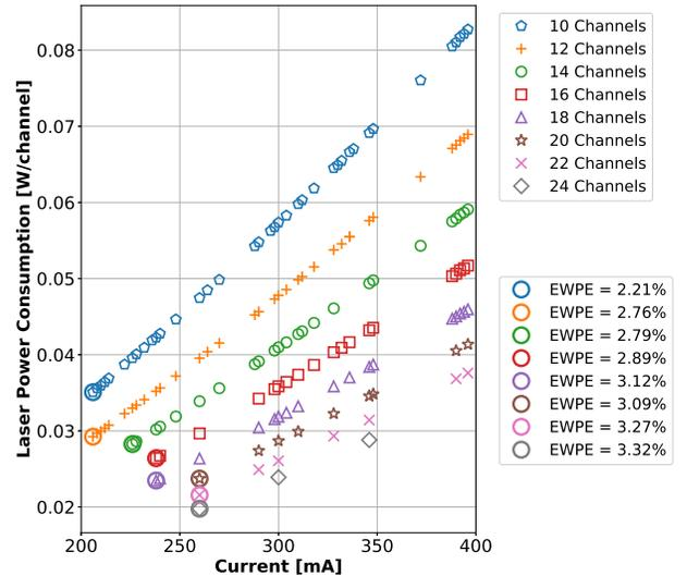
Figure 2. Dependence of Innolume comb laser total electrical power per channel on current for various channel counts with a fixed channel spacing and a  $\mathcal{P}_b = 0 \text{ dBm}$ . Circled points indicate optimal energy efficiency for each channel count with respective EWPE values.
